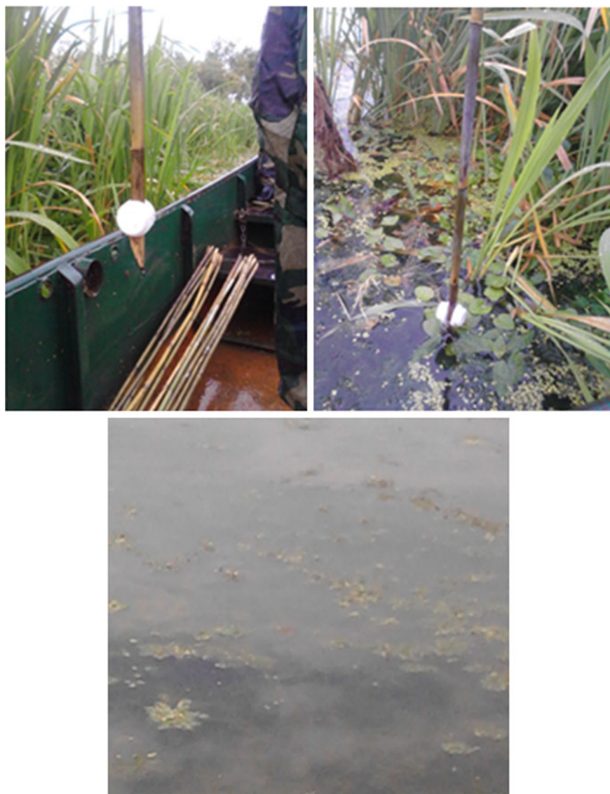
Fig. 7.1 The insertion operation of DGT pistons into the rhizosphere of Zizania caduciflora and Myriophyllum verticillatum
