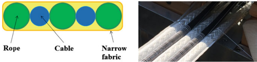
Fig. 2 Schematic cross section illustration ( left ), fabric composite for preliminary tests ( right ) [1, 2]
