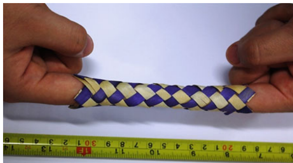
Fig. 1 Braided ‘Chinese finger trap’ that uses the principle of strand shearing under tension
