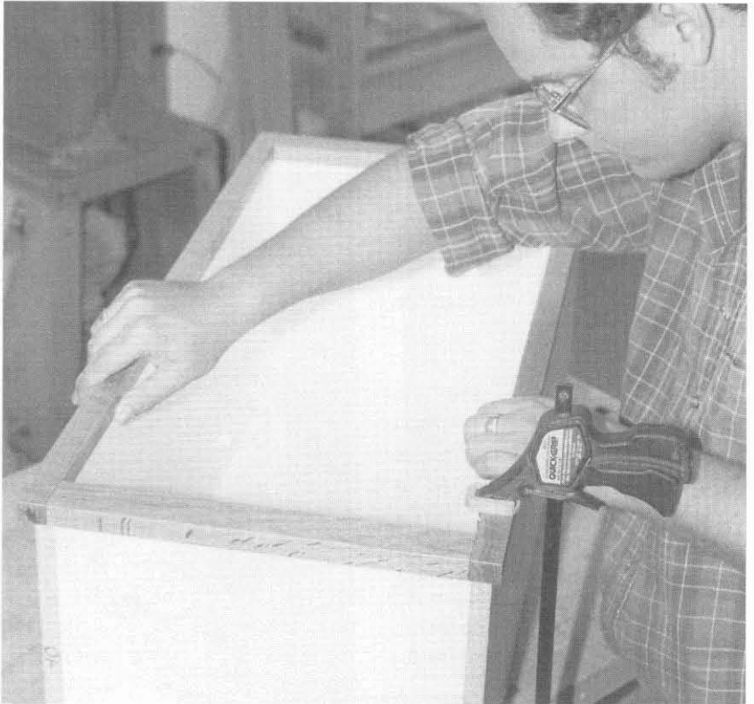
Installing the face frame flush with the inside face of the cabinet's side board is another common building practice.
