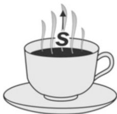
Fig. 3.1 Entropy in everyday life: Generally stated, it is that which hot coffee loses when it cools down in a cup and what is added to a pot of soup to heat the food. It is what is generated in a hot plate, a microwave oven, and an oil heater. Entropy is also what is transported in hot water and distributed by a radiator. It is what is conserved by the insulating walls of a room and by the wool clothing worn by the body.
