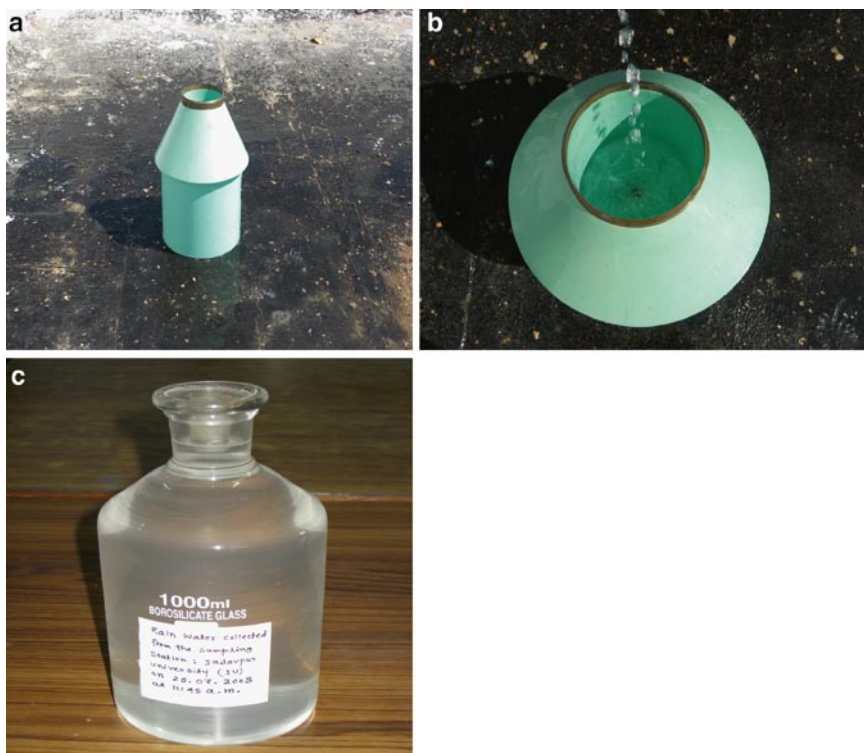
Fig. 7.3 (a) Bucket used for rainwater collection. (b) Collection of rainwater. (c) Rainwater stored in a reagent bottle for analysis
