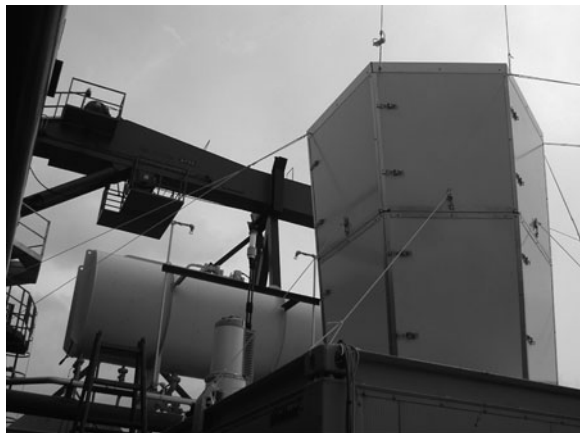
Fig. 1 The ZephIR wind LiDAR in the centre of the image and the AQ500 SoDAR in the front right installed at the Horns Rev platform in 2006
