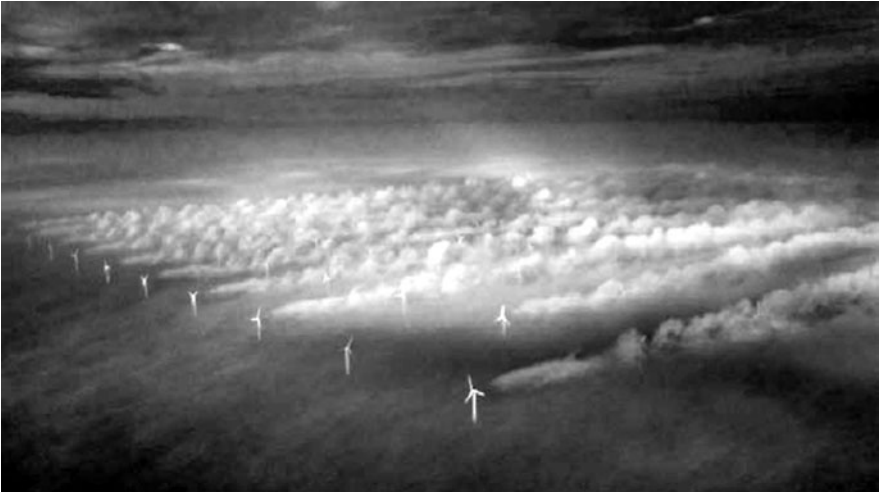
Fig. 5 An offshore farm of wind turbines with their array interference effects being identified by natural condensation of water vapor in their downstream wakes. Source: Uni-Fly A/S, Vattenfall windkraft, Erik Slot, BWEA Offshore 08, Westminster, June 4, 2008
