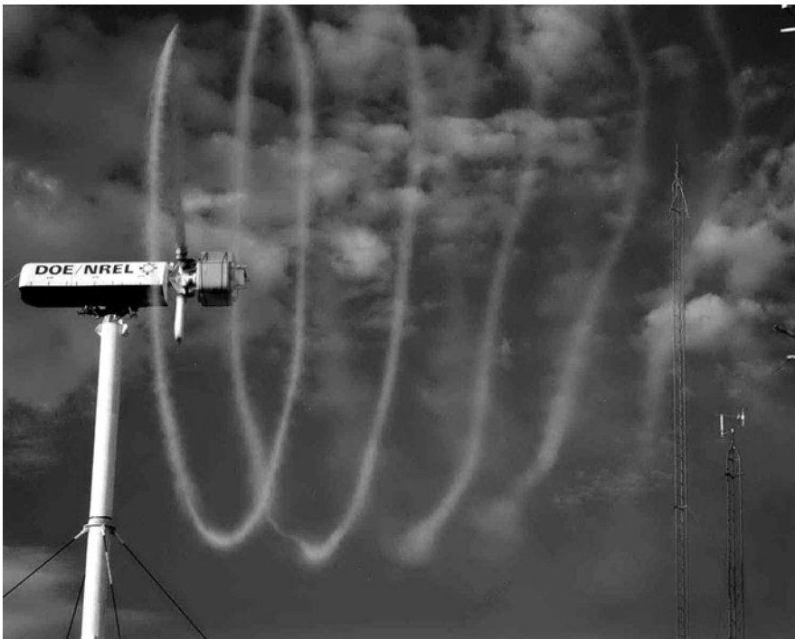
Fig. 28 Photograph of the vortical wake behind a downwind type of HAWT rendered visible using smoke injection from smoke “bombs” placed at the blade tips (photo courtesy of NREL)
