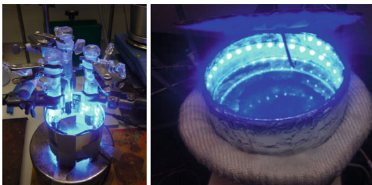
Fig. 3 Homemade visible-light batch reactors with LED strips lining the inside of cylindrical containers. Images reprinted with permission from Weiss et al. [21] (left) and Senaweera et al. [22] (right)
