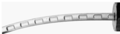
Fig. 1 Gas/liquid segmented flow pattern for the oxidation of cyclohexane with air. Reproduced with permissions from [41]
