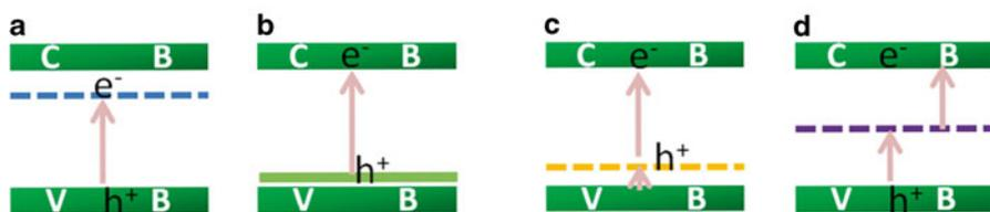
**Fig. 19.3** Four proposed schemes illuminating the possible origin of visible light absorption and enhanced photocatalytic activity in doped BiOX: (a) self-doping: introduction of defect states below conduction band (CB); (b) alloyed effect: introduction of hybridization of the halogen np states on the top of valence band (VB); (c) nonmetal doping: introduction of impurity level above valence band; (d) metal doping: introduction of localized energy levels above valence band
