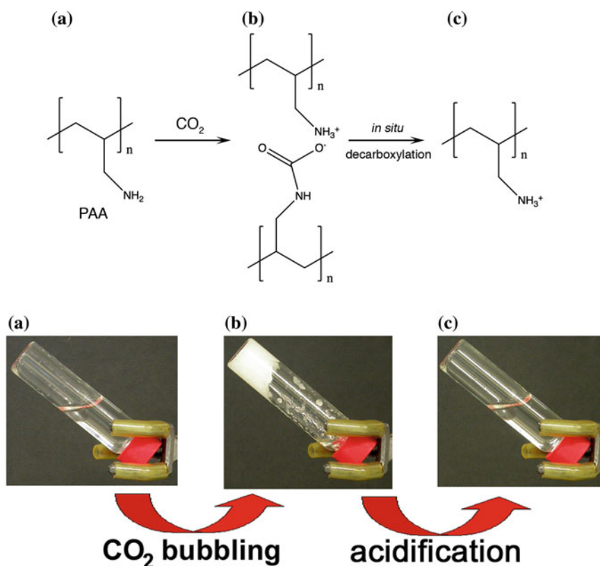
Fig. 7 Mechanism of formation of a polyallylamine rheoreversible gel: bubbling \text{CO}_2 into solution leads to gel formation, while acidification converts the gel back to a free-flowing system. (Reprinted with permission from Carretti et al. (2004). Copyright (2004) American Chemical Society)
