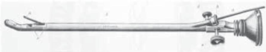
Fig. 10. Maximilian Nitze's cystoscope, showing the probe channel, urethral probe, and bulb illumination.
