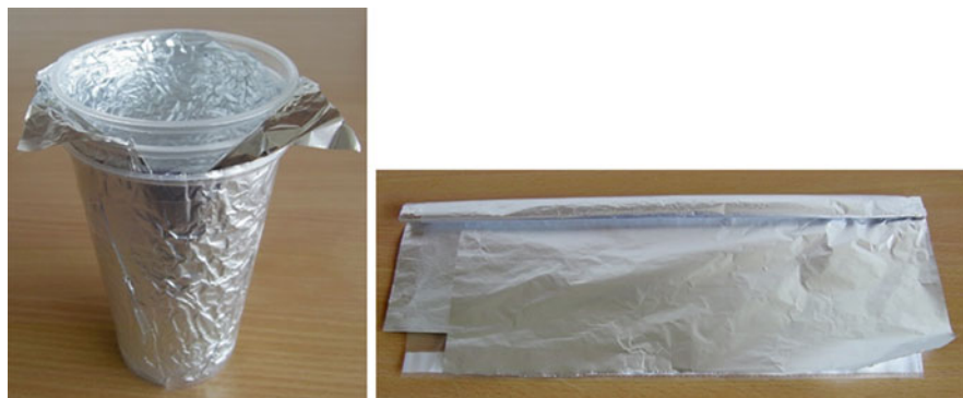
Fig. 16.8 Capacitor from cups (left) and from aluminium and plastic foils (right)
