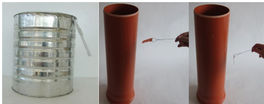
Fig. 16.1 Arrangement of the experiment—charged tin (left) and charged place (middle) and place without charge on a plastic tube (right)
