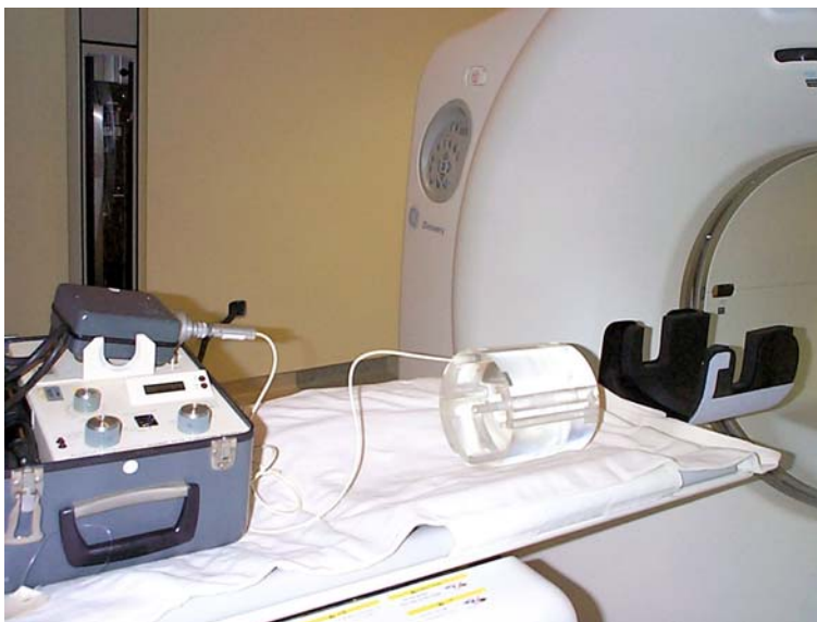
Fig. 19.1 A typical setup of the dosimeter, ionization chamber, and 16-cm diameter acrylic phantom for measuring the CTDI of the head. There are four holes 1 cm from the surface and one hole in the center of the phantom for insertion of the ionization chamber for dose measurements
