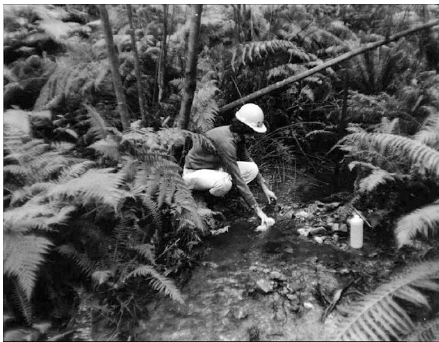
Fig. 9.1 Taking a manual water sample in a first order stream. There is not much water depth to play with. This, the most primitive technique in water quality measurement, is still fundamental
