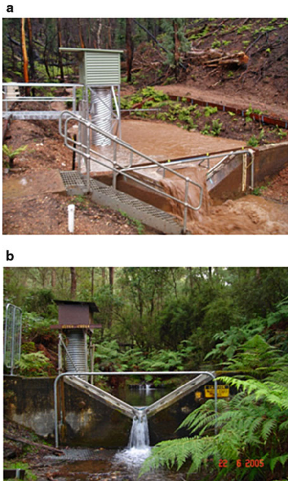
Fig. 9.2 Extremes of water quality at Croppers Creek (a) Clem Creek after fire with high flows and an associated very high turbidity and (b) Betsy Creek 18 months before the fire with very high water quality. The turbidity of this water is at the lowest end of naturally-occurring waters
