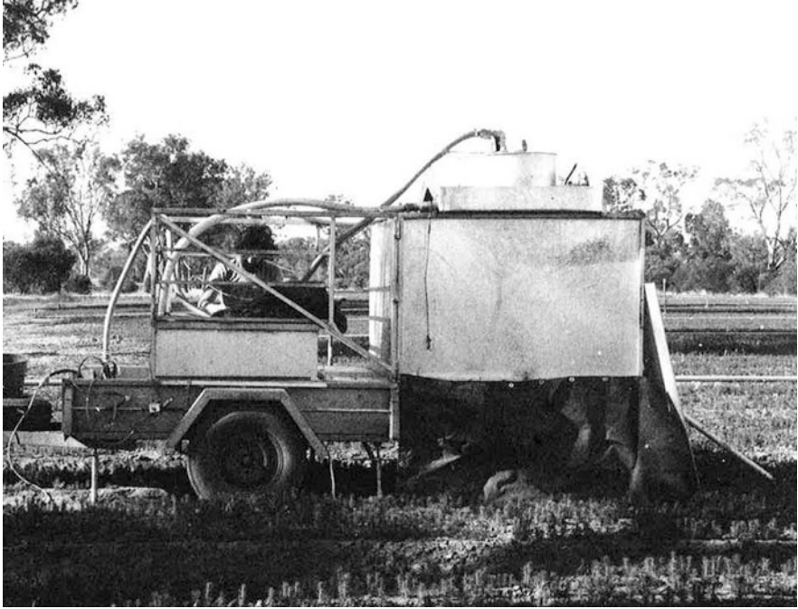
Fig. 4.7 Use of a sprinkling infiltrometer in a study of the impact of soil slaking on infiltration into a nursery soil. Water is pumped from a storage tank to the rotating disc on top, from where it “rains” onto a bounded plot. It worked well on agricultural soils but could not meet the high infiltration capacity of forest soils
