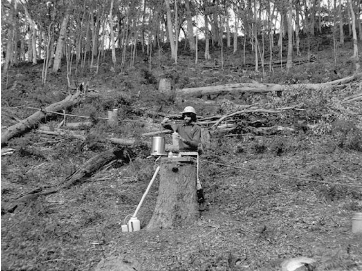
Fig. 2.4 Locating a rain gauge in a clearing in a forest usually involves a lot of cutting. This (just) gave a 30° cone of clearance. To the far right is a standard 203 mm storage gauge. A tipping bucket gauge sits on a convenient stump. The cable carries the data to a nearby data logger. Technician Leon Stephens is decanting a rainfall sample collected in the storage bottle on the ground for chemical analysis (see Hopmans et al. 1987)
