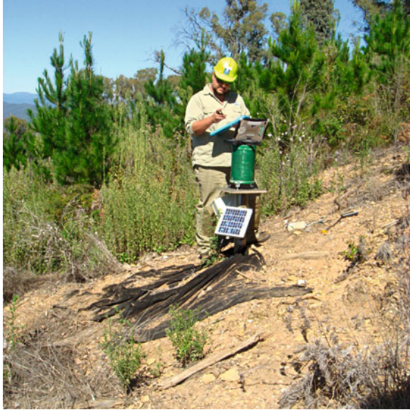
Fig. 2.1 Technical officer John Costenaro downloading a recording rain-gauge in a study of rainfall distribution on the burnt Clem Creek catchment
