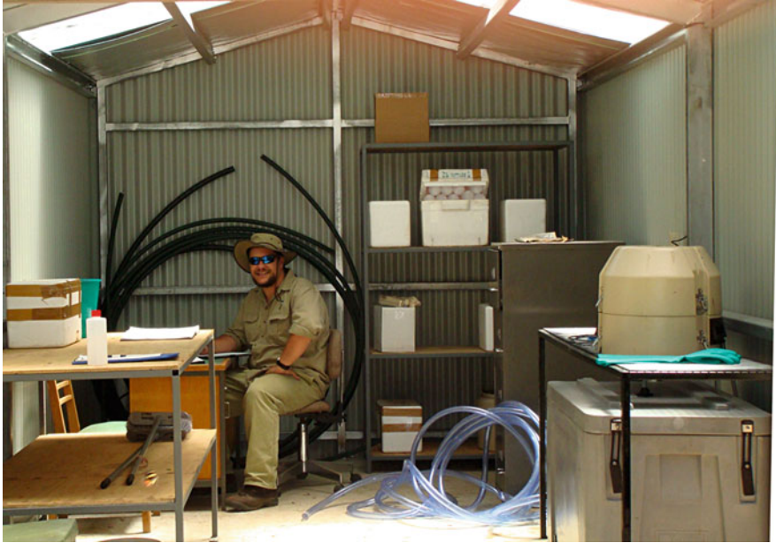
Fig. 9.5 A sophisticated water sampling setup at Ella Creek weir. To the right is a data-logger-controlled water sampler. Samples pass into a bulk container to give an “average sample” for a given period. Shelves allow storage of containers, hoses, etc. Technical officer John Costenaro is seen doing the never-ending paper work associated with running a water-sampling program. The ability to do the routine work protected from the weather adds greatly to the quality of such programs
