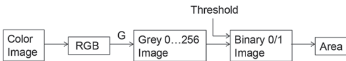
Fig. 9.3 Image segmentation for size feature extraction. (Reprinted with permission from Martynenko 2011. © 2008 Springer)
