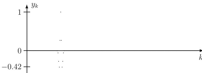
Fig. A.24 Data according to Fig. 5.17, processed with the modified high-pass filter according to (A.4). The undershoots get a bit smaller and wider. Progress admittedly is small, yet visible
