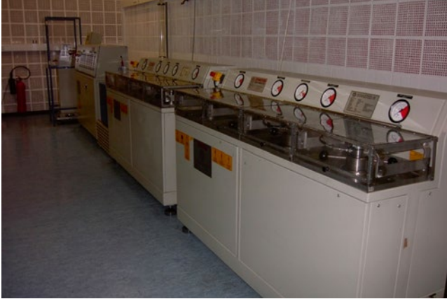
Fig. 3.12 Multi-vessel system 8 vessels
