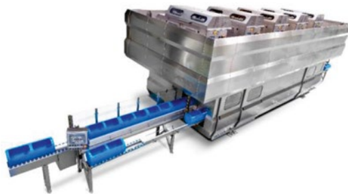
Fig. 3.4 Hiperbaric 525 equipment: vessel volume of 525 L, integrated design with five high-pressure pumps including double intensifiers on the top of the vessel, carriers loading and unloading lines, carrier return line, and operator panel. Maximum working pressure: 600 MPa (87,000 psi)
