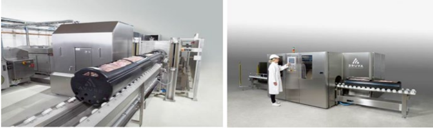
Fig. 3.2 Commercial-scale high-pressure equipment system (horizontal configuration)
