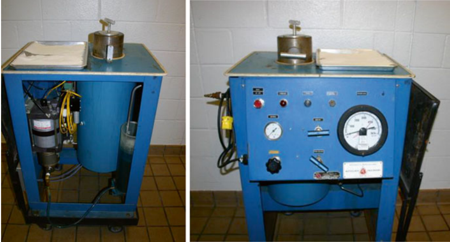
Fig. 2.1 Autoclave Engineers CIP 2-22-60 isostatic press at Oregon State University
