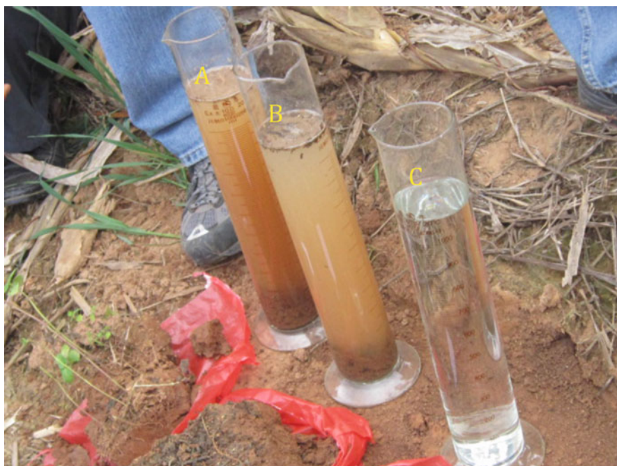
Fig. 8.1 An experiment comparing the stability of natural (forest) soil ( b ) and cultivated soil ( a ). Procedure: (1) Use three test tubes, filled with water to three fourths of length; (2) collect soil from cultivated field ( C ) and from forest area ( F ); (3) grind soil and remove plant debris; (4) put 50 g soil from C and F into test tubes ( a and b , respectively), stir for 1 min with rod or spoon; (5) compare color of soil solutions after 5 min. Result: Most of the soil in test tube a is dissolved making the solution opaque, but it is opposite in test tube b , where most of the soil is deposited at the test tube bottom. Test tube c is the control (water only)
