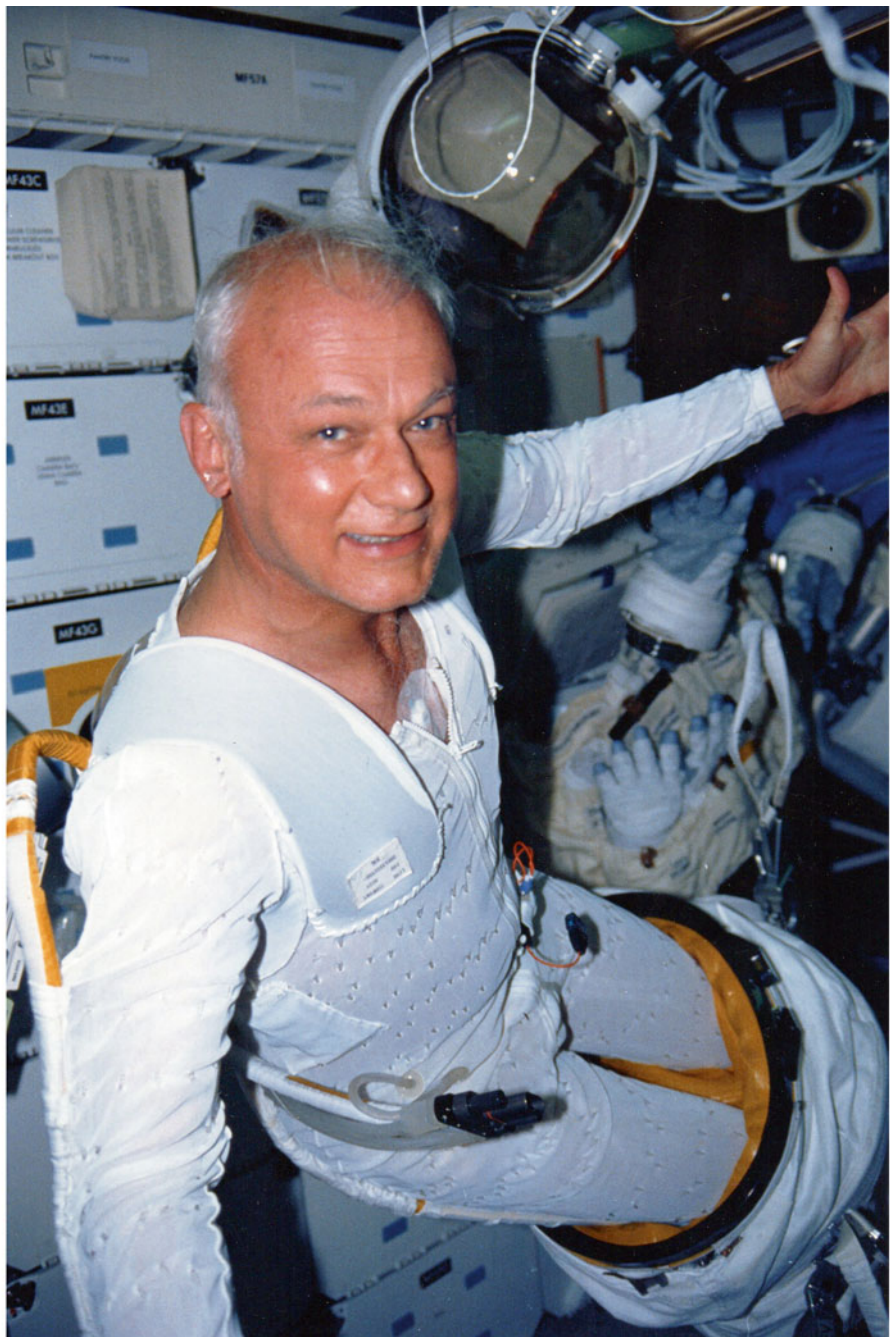
Bruce McCandless with his legs partially in the lower torso of an EMU, wearing the liquid coolant undergarment. His helmet and gloves float behind him.
