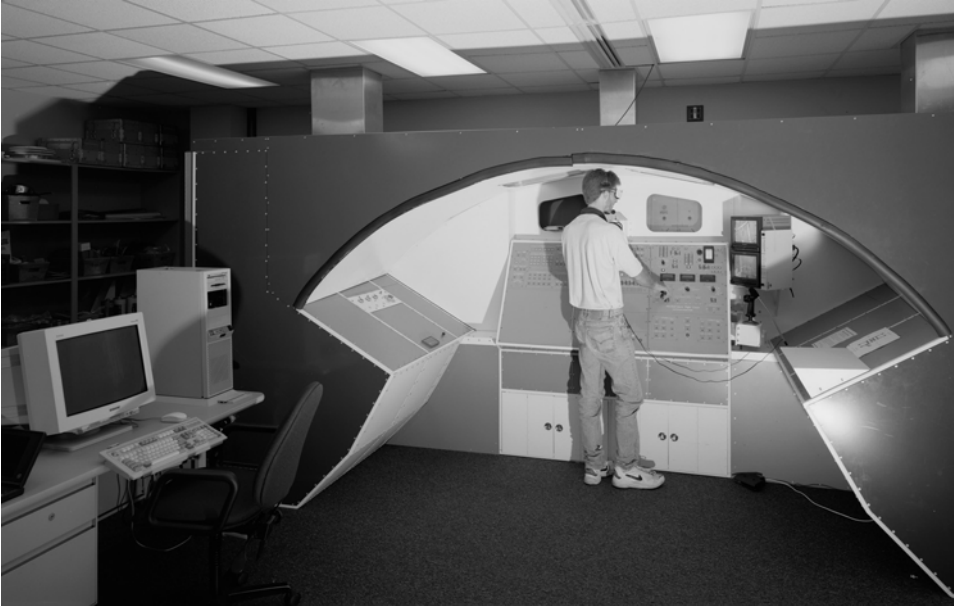
The NBS RMS simulator control room at MSFC reproducing identical RMS controls and panels to the shuttle orbiter aft flight deck. Wearing glasses, an operator could view 3-D video projection in the aft flight deck windows as the operator could not view operations in the water tank while at the control panel. (Courtesy NASA MSFC History Office/US Library of Congress Historic American Building Collection; HAER ALA,45-HUVI.V,7B-14; 1995, by Jet Lowe)
