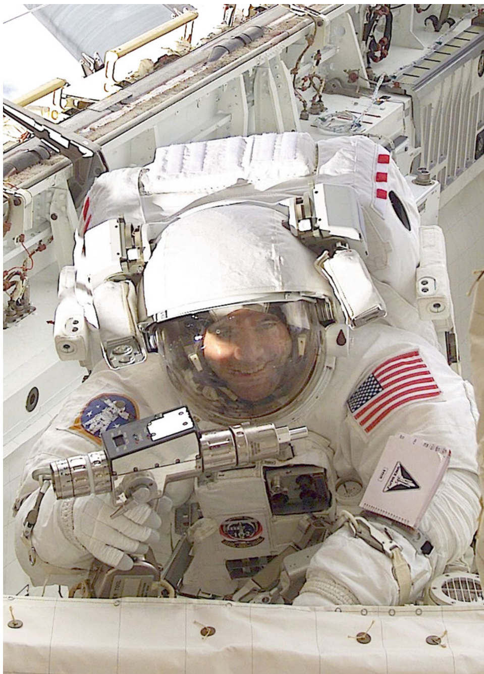
Paul Richards putting his design for a pistol grip tool through its paces during an EVA on the ISS assembly mission on STS-102.
