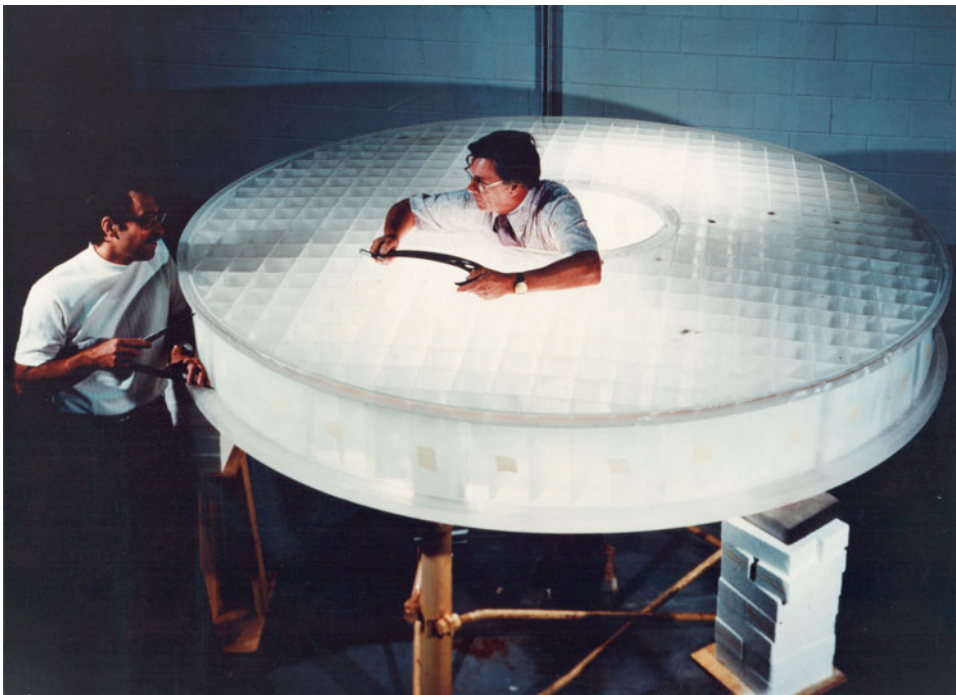
Primary mirror construction.
