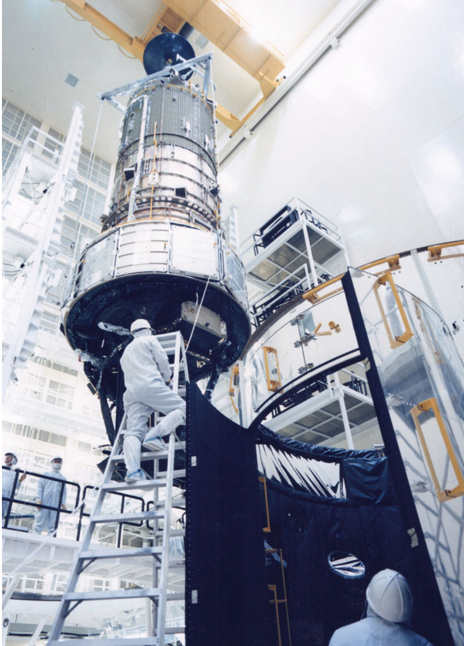
The Optical Telescope Assembly is lowered into the Aft Shroud. (Courtesy British Interplanetary Society)
