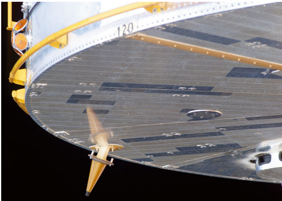
Close up view of the base of Hubble showing one of the low gain antennas and circumferential EVA hand rails.
