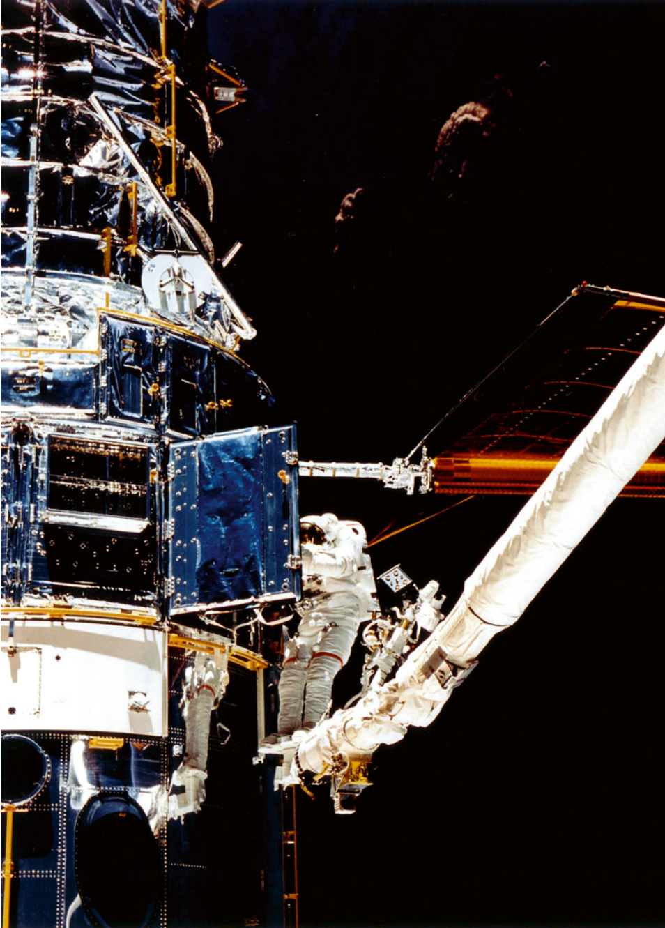
Jeff Hoffman, high above the payload bay, works on changing Hubble's fuse plugs during the first EVA.
