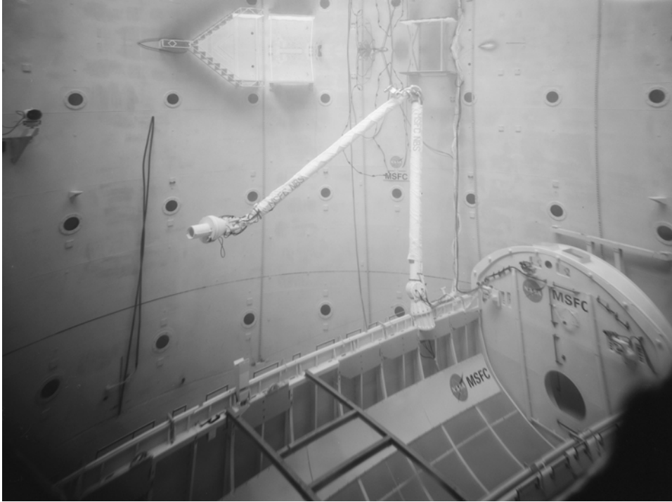
The RMS simulator in the NBS tank at Marshall Space Flight Center. (Courtesy NASA MSFC History Office/US Library of Congress Historic American Building Collection; HAER ALA,45-HUVI.V,7B-11; 1995, by Jet Lowe)
