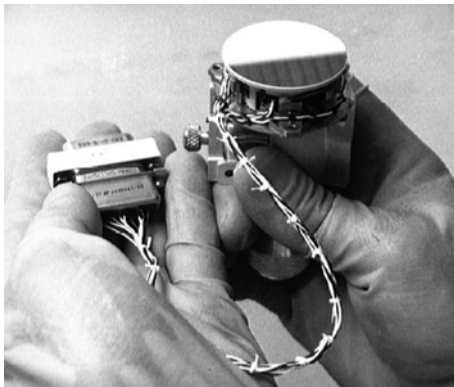
The tiny mirrors of the COSTAR package for Hubble ( left ) and the light path in the WFPC using the corrective optics.
