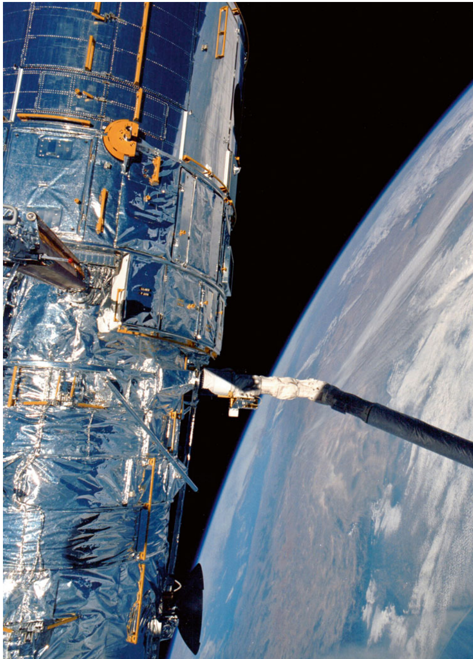
Discovery's Remote Manipulator System (RMS) is shown attached to Hubble high above the Earth. Yellow handrails, foot restraint attachment points and insulation covering are clearly visible.
