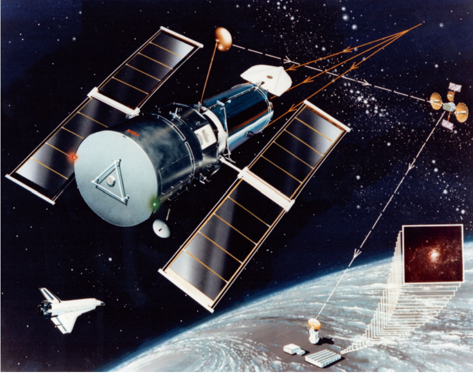
Space Telescope communications links through a Tracking and Data Relay Satellite (TDRS). (Courtesy British Interplanetary Society)
