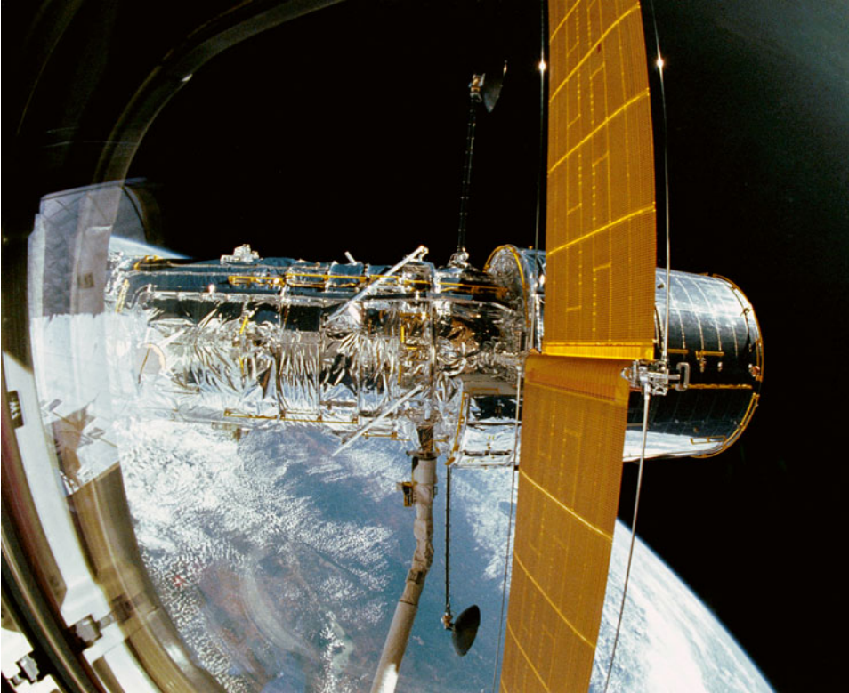
Hubble on the end of the RMS seen through the overhead aft flight deck windows.
