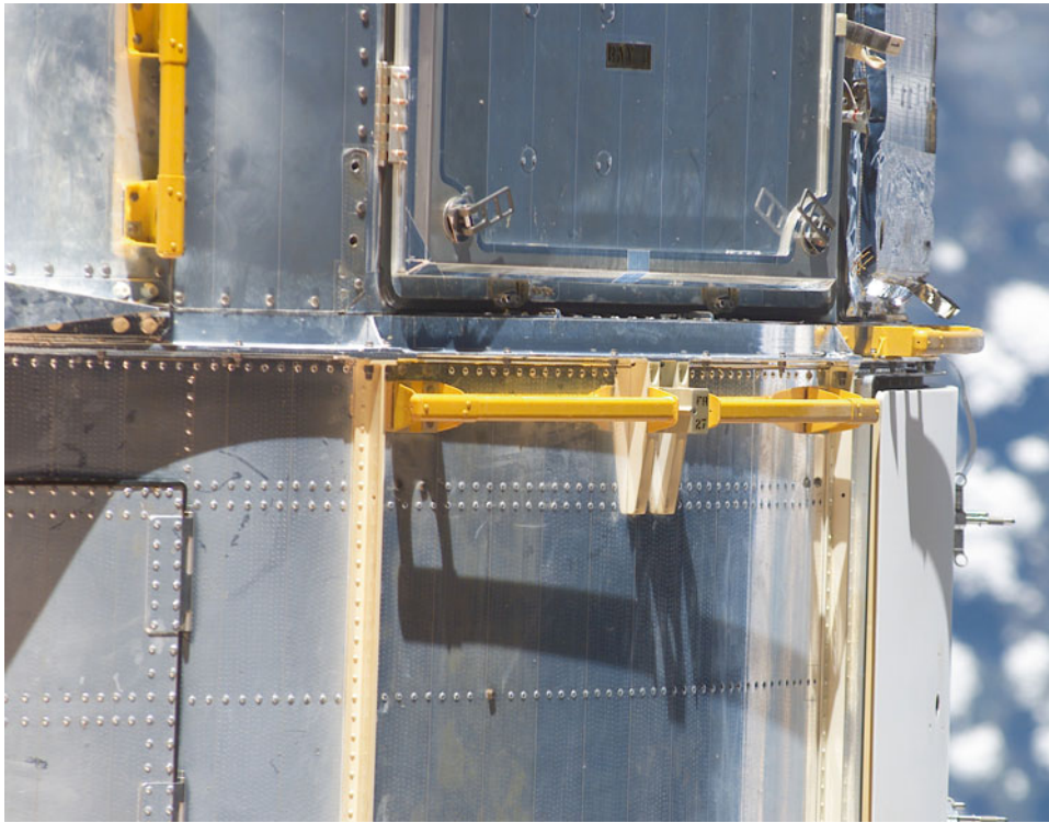
Close up view of the EVA handrails across the Hubble Telescope structure.
