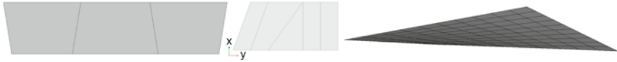
Fig. 5.4 Quadrilateral elements with mesh quality exceed the minimal in-house recommended values of a Jacobian of 0.7 ( left ), internal angle of 55, 10^\circ exceed the recommended 45^\circ ( center ), and a warpage of 1.65 ( right )
