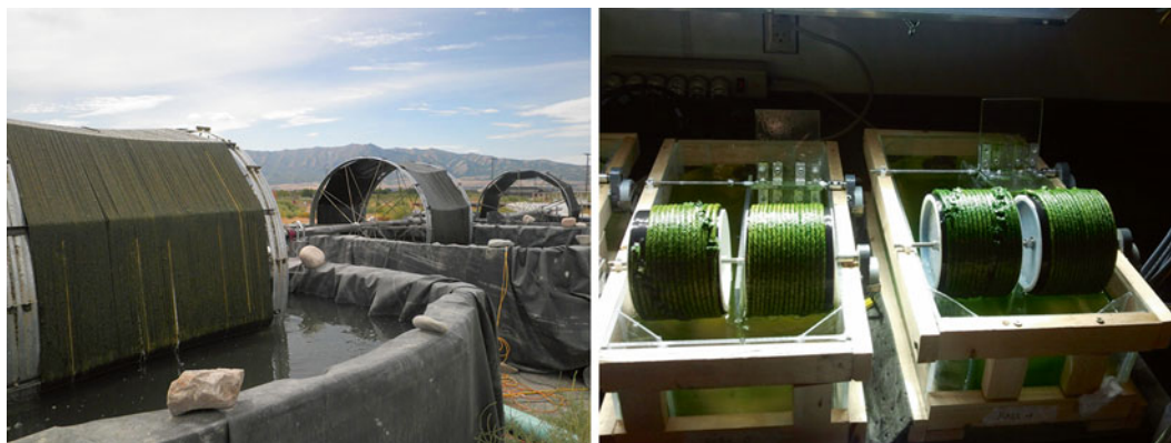
Fig. 3.1 Pilot and laboratory-scale rotating algal biofilm reactors (RABR) for treating wastewater effluent from Logan City sewage lagoons and providing biomass for bioproducts (Courtesy of the Sustainable Waste-to-Bioproducts Engineering Center (SWBEC), Utah State University)
