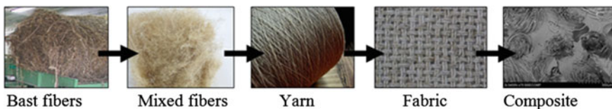
Fig. 6 Scheme of technological chain of bast fibers and fabric application to composite
