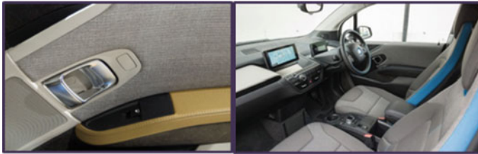
Fig. 11 Elements of BMW i3 made of composites reinforced with kenaf [86]
