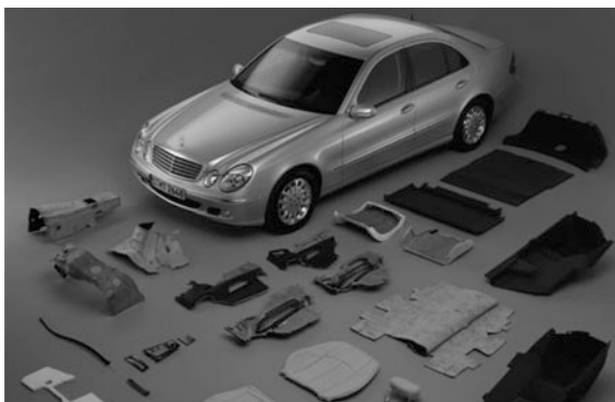
Fig. 9 Flax, hemp, sisal, wool, and other natural fibers are used to make 50 Mercedes Benz E-Class components [83]
