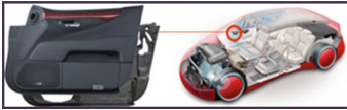
Fig. 10 Door trim using material made from kenaf and PLA [85]
