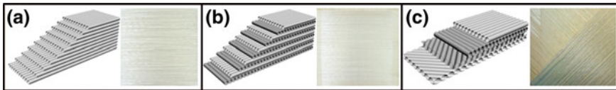
Fig. 9 a Unidirectional non-interlaced fabric schematic and actual fabric. b Biaxial non-interlaced fabric schematic and actual fabric. c Multi-axis non-interlaced fabric schematic and actual fabric [25]
