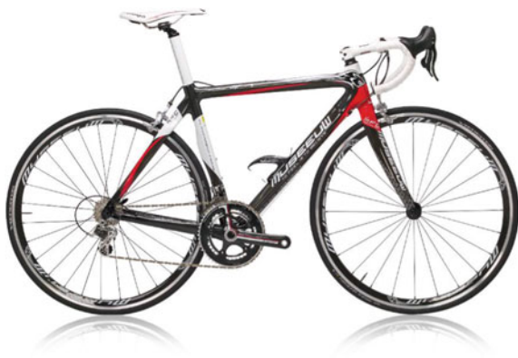
Fig. 13 Bicycle with frame made of flax-carbon composite [89]
