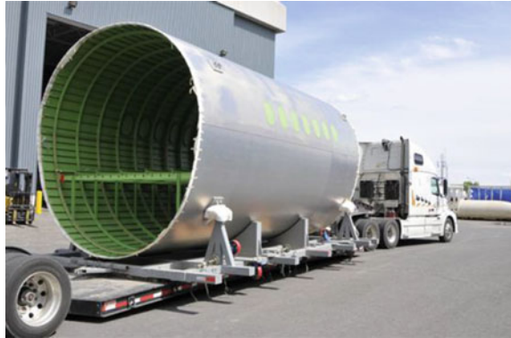
Fig. 8 Picture showing Bombardier C series Fuselage—GLARE. Ref. [37]
