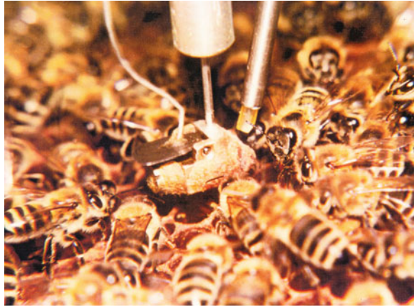
Fig. 17.3 A mechanical robot model of a dancing honeybee photographed during its performance of a waggle dance among the bees on the dance floor of an opened observation hive. A number of bees are facing the robot and running along with it, and some of these bees later appear at the location indicated by the robot's dance (from Michelsen et al. 1992)
