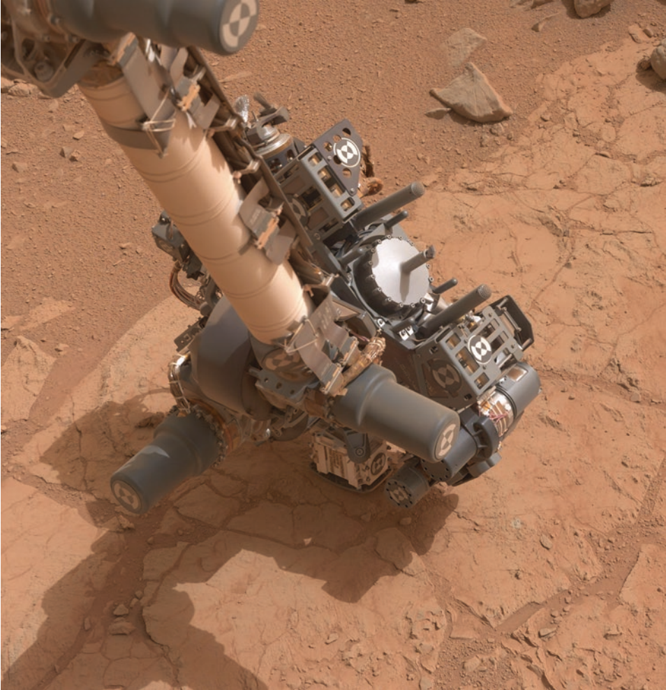
Figure 9.8. APXS deployed onto the John Klein drill target. Mosaic of four Mastcam images taken on sol 168. Credit: NASA/JPL-Caltech/MSSS.
