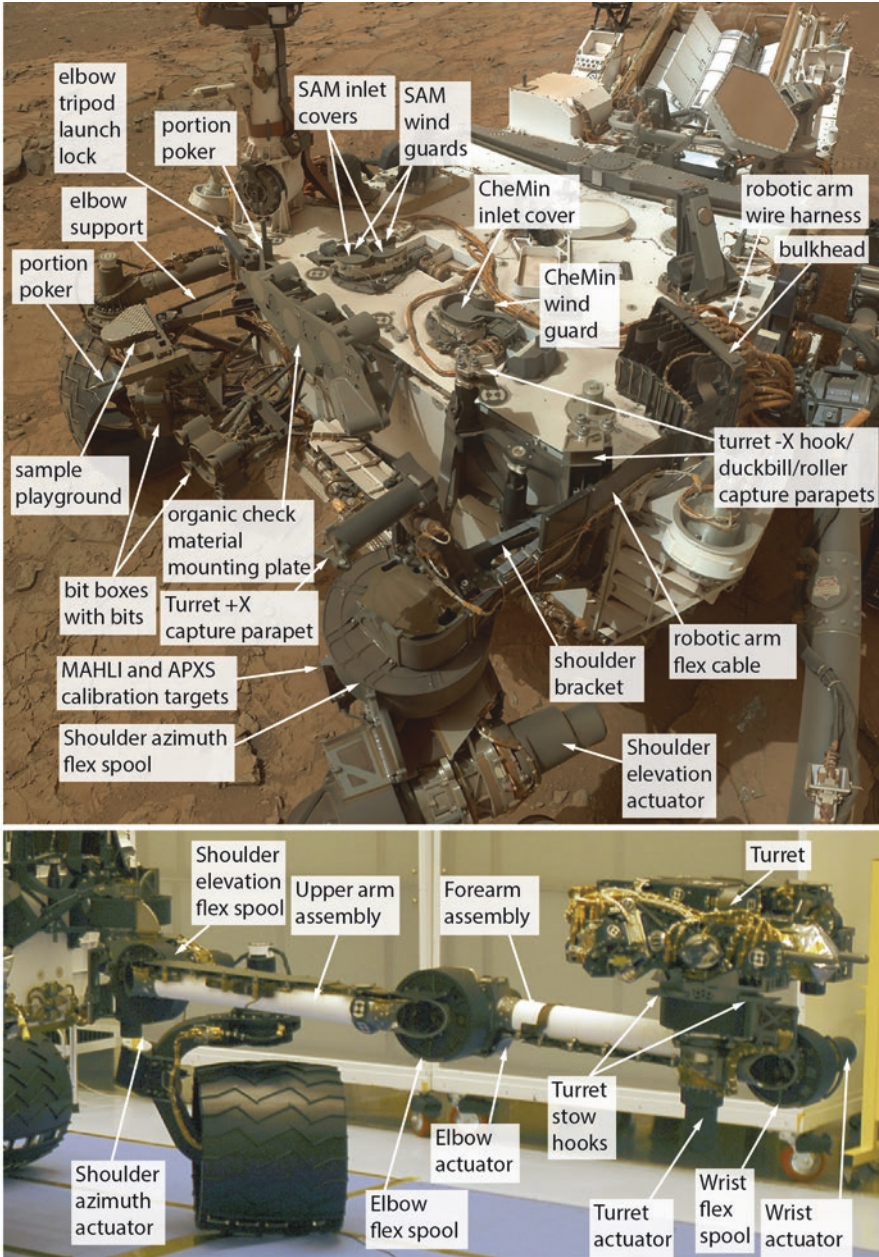
Figure 5.1. Parts of Curiosity's Sample Acquisition, Processing, and Handling (SA/SPaH) system. Top image is the John Klein self-portrait from sol 177 (NASA/JPL-Caltech/MSSS); bottom image was taken during testing at Kennedy Space Center on August 13, 2011 (NASA release KSC-2011-6470), annotated by Emily Lakdawalla.
