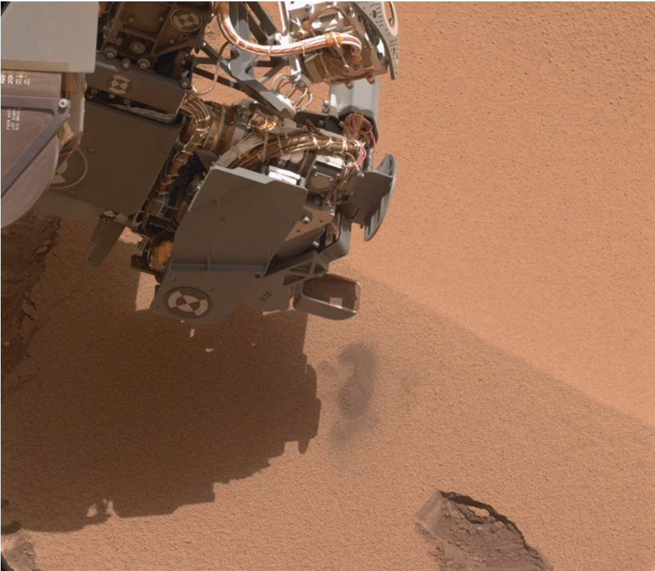
Figure 3.6. Left Mastcam photo 0061ML0003060000102375E01 documenting the first day of scooping at Rocknest. CHIMRA acquired a full scoop from the site at lower right, then shook out some of the sample to reduce the amount in the scoop, leaving a fresh pile of dark sand on the ripple surface. NASA/JPL-Caltech/MSSS.
