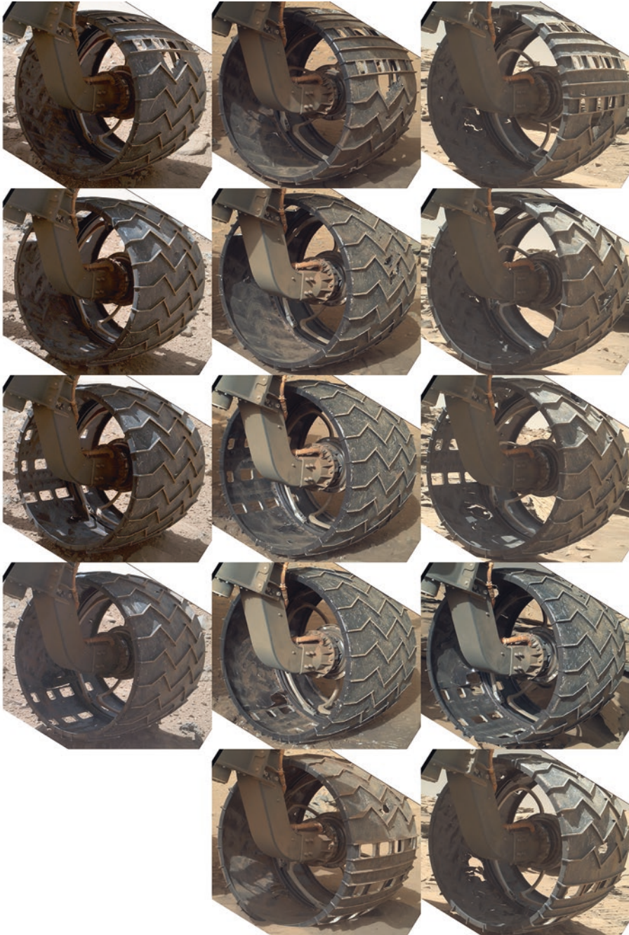
Figure 4.22. MAHLI survey of left front wheel on sol 513 (left column), 708 (middle), and 1313–1315 (right). See text for discussion. NASA/JPL-Caltech/MSSS.
