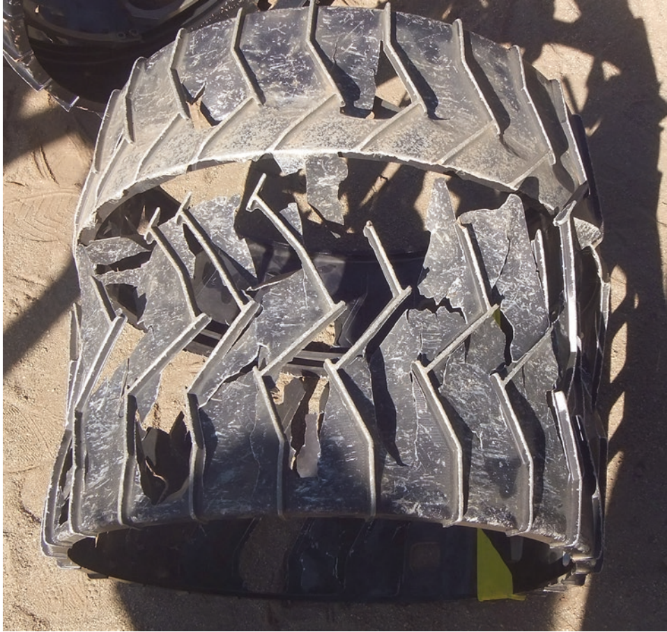
Figure 4.23. Wheel tested to failure. The rover can still drive effectively on this wheel, but the sharp edges of the broken grousers and webbing present a hazard. Photo taken in the JPL Mars Yard on October 13, 2014 by Emily Lakdawalla.
