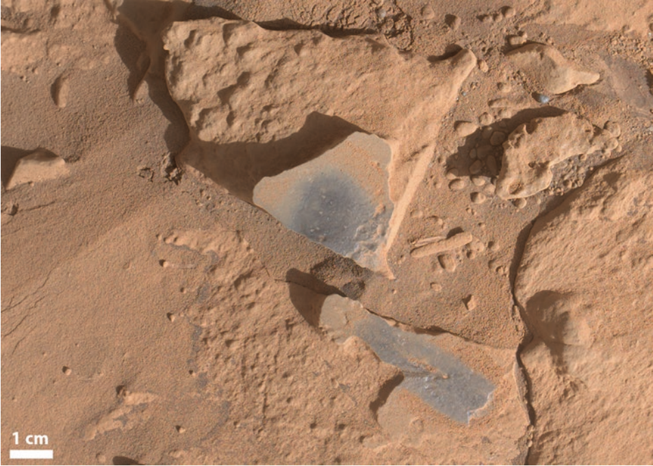
Figure 9.7. Two ChemCam raster targets at Windjana, “Stephen” (top) and “Neil” (bottom), were dusted off by ChemCam, revealing the dark color of the rock beneath the bright dust. MAHLI image 0627MH0001900010203555C00, NASA/JPL-Caltech/MSSS.
