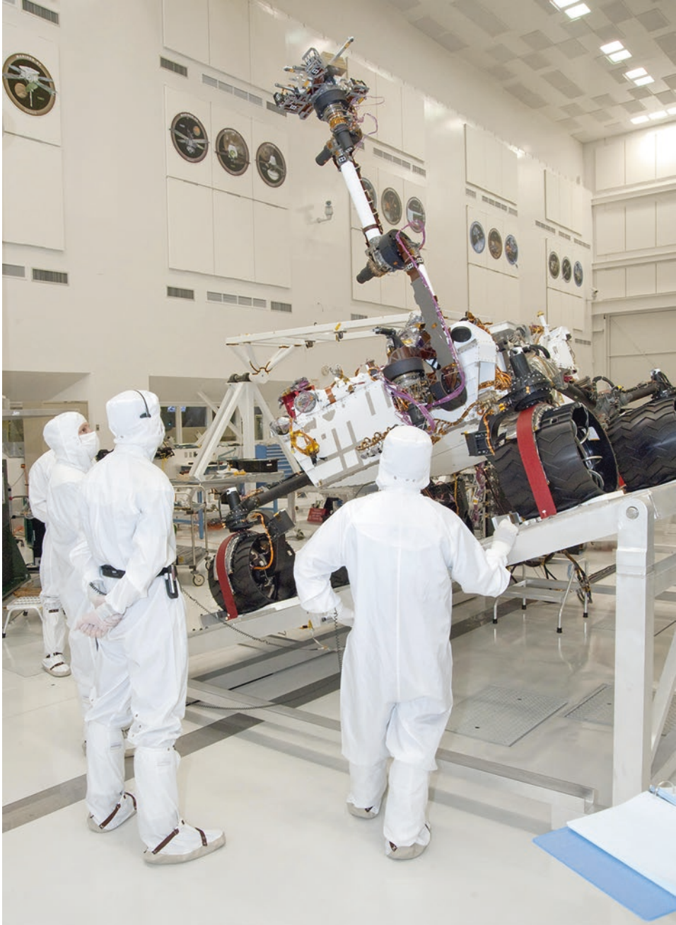
Figure 1.19. Testing out the arm's positioning from a tilted rover, 16 September 2010. NASA/JPL-Caltech release PIA13389.
