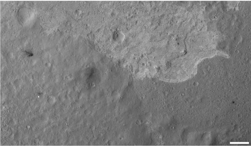
Figure 2.35. HiRISE image of the MSL landing site, sol 1 (August 7, 2012). The impact sites of the backshell, descent stage, and parachute are to the left of the blast zone that marks the rover, uprange; the heat shield is downrange, to the right. HiRISE image ESP_028269_1755. NASA/JPL-Caltech/UA.
