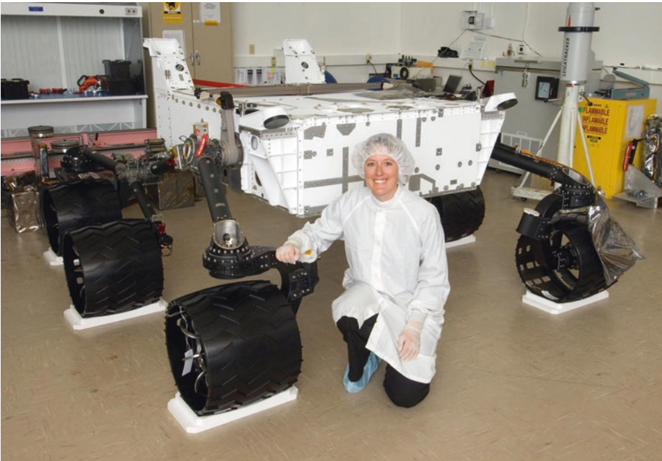
Figure 1.12. The mobility system was attached to the flight model of the rover in August 2008. NASA/JPL-Caltech release PIA11438.
