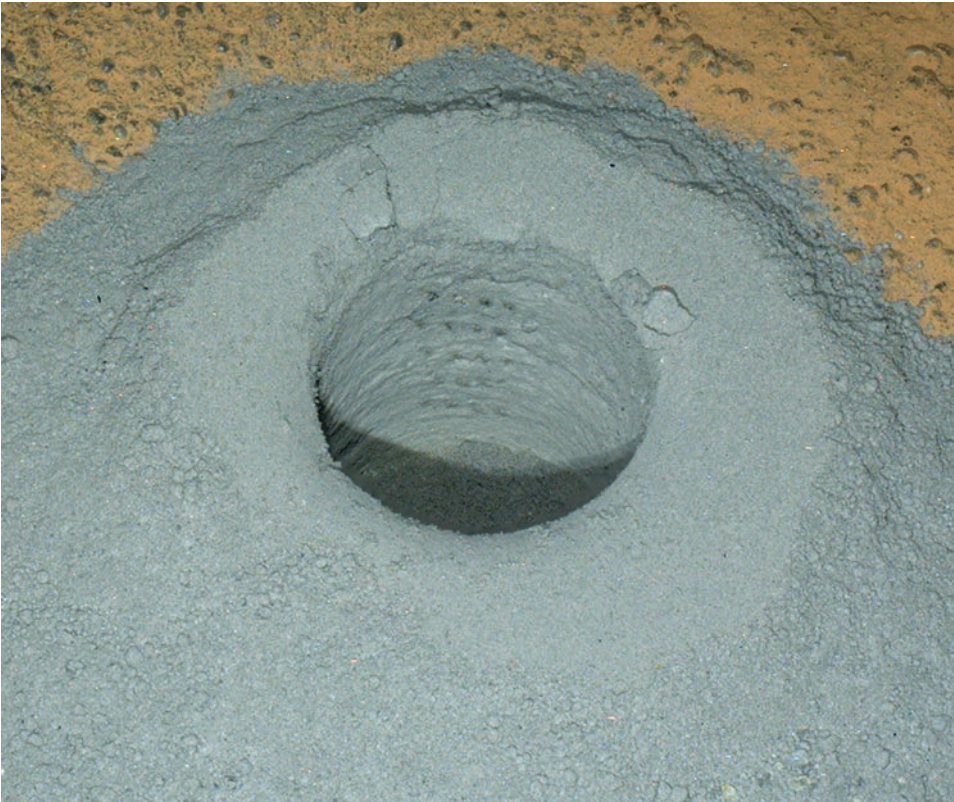
Figure 6.2. ChemCam laser shots are spaced using minute motions of the remote sensing mast. Here, ChemCam laser shots are spaced 1.4 mm apart horizontally in rasters marching down the wall of the Okoruso drill hole. Drill holes are 1.6 centimeters in diameter, and this one was 2.6 meters away from the mast head when the shots were fired. Corresponding mast shot-to-shot angular motion was 0.03^\circ (0.5 milliradians). MAHLI image 1338MH0005880000501506R00, taken at night with LEDs on. Contrast in the image has been increased to emphasize the laser shot points. NASA/JPL-Caltech/MSSS/Emily Lakdawalla.
