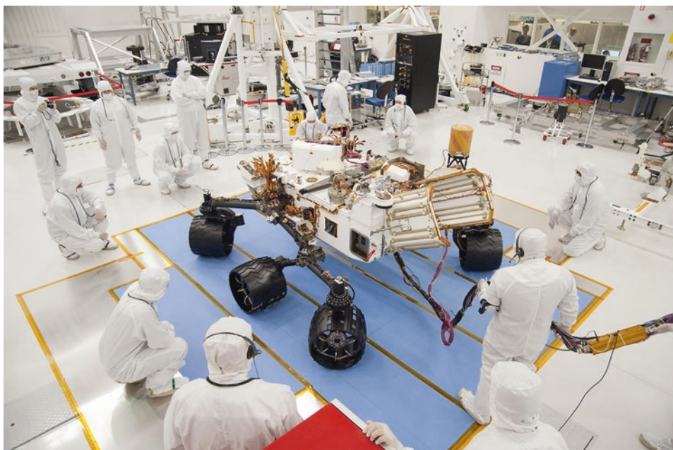
Figure 1.18. The rover's first drive, 23 July 2010. The corner wheels are steered into position to allow the rover to turn in place. NASA/JPL-Caltech release PIA13308.
