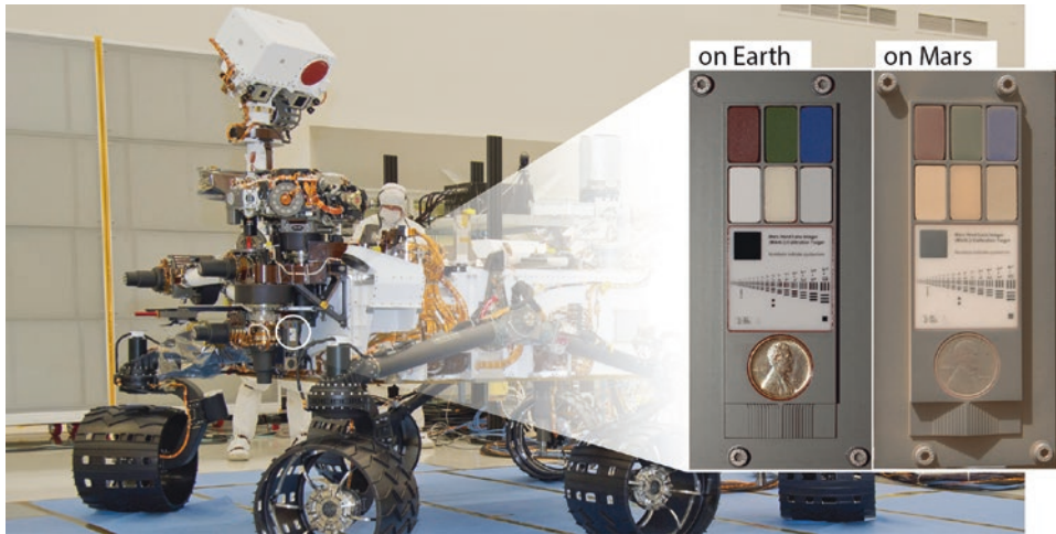
Figure 7.13. Photo of the rover taken during assembly at JPL, showing the location of the calibration target. NASA/JPL-Caltech release PIA14289. Insets: two images of the calibration target, taken before departing Earth using a DSLR camera (left) and after landing on Mars, by MAHLI (right). Image 0034MH0000460010100041E01. NASA/JPL-Caltech/MSSS/Emily Lakdawalla.
