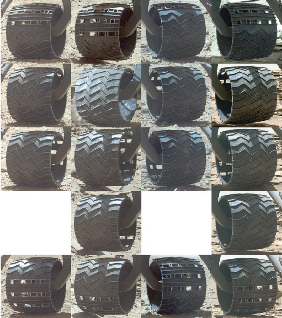
Figure 4.20. MAHLI survey of rear wheels on sols 513 and 1313–1315. See text for discussion. NASA/JPL-Caltech/MSSS.
