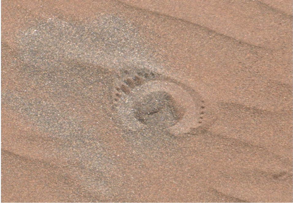
Figure 9.12. The APXS “nose print” in the fine sand at Gobabeb as seen from Mastcam. The inner, open circle of the APXS contact plate is 29 millimeters in diameter. Mastcam image 1234MR0057070010603445E01. Credit: NASA/JPL-Caltech/MSSS.
