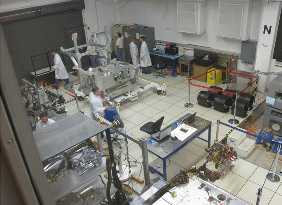
Figure 1.11. Testbed rover hardware in the In-Situ Instrument Laboratory at JPL, August 25, 2008. The aluminum box at top center is the rover body. The mobility system is at left, with wheels behind red ropes at right. Arm hardware is at the bottom right. Photo by Emily Lakdawalla.
