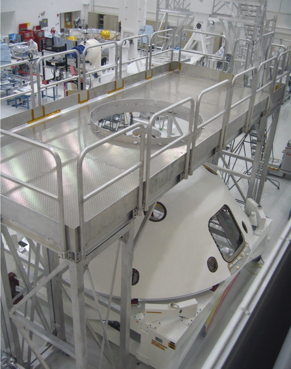
Figure 1.14. In the foreground, MSL's gargantuan backshell, with its human-scale access port that would later be used for MMRTG installation, covered with a custom-built aluminum platform for work access. Behind it, an enormous (and enormously expensive) rotisserie-type rig upon which the spacecraft could be stacked and inverted. In the background, the cruise stage comes together. October 16, 2008. Photo by Emily Lakdawalla.
