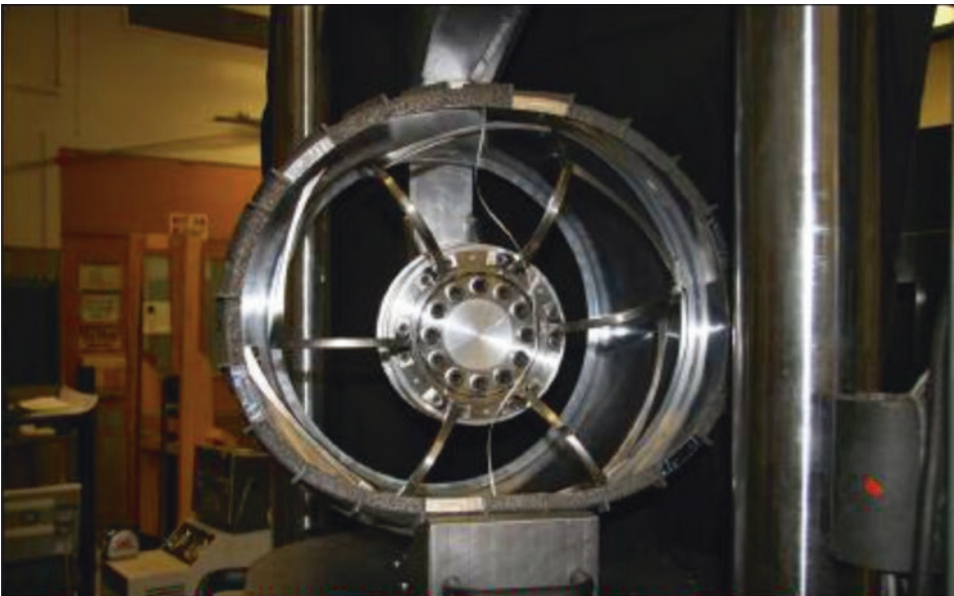
Figure 4.15. Spring-like deformation of a rover wheel during testing. In this test, two of the spokes have “bottomed out” on the inside surface of the wheel. After this test, the wheels sprang back to their original shape. From Lee (2012).
