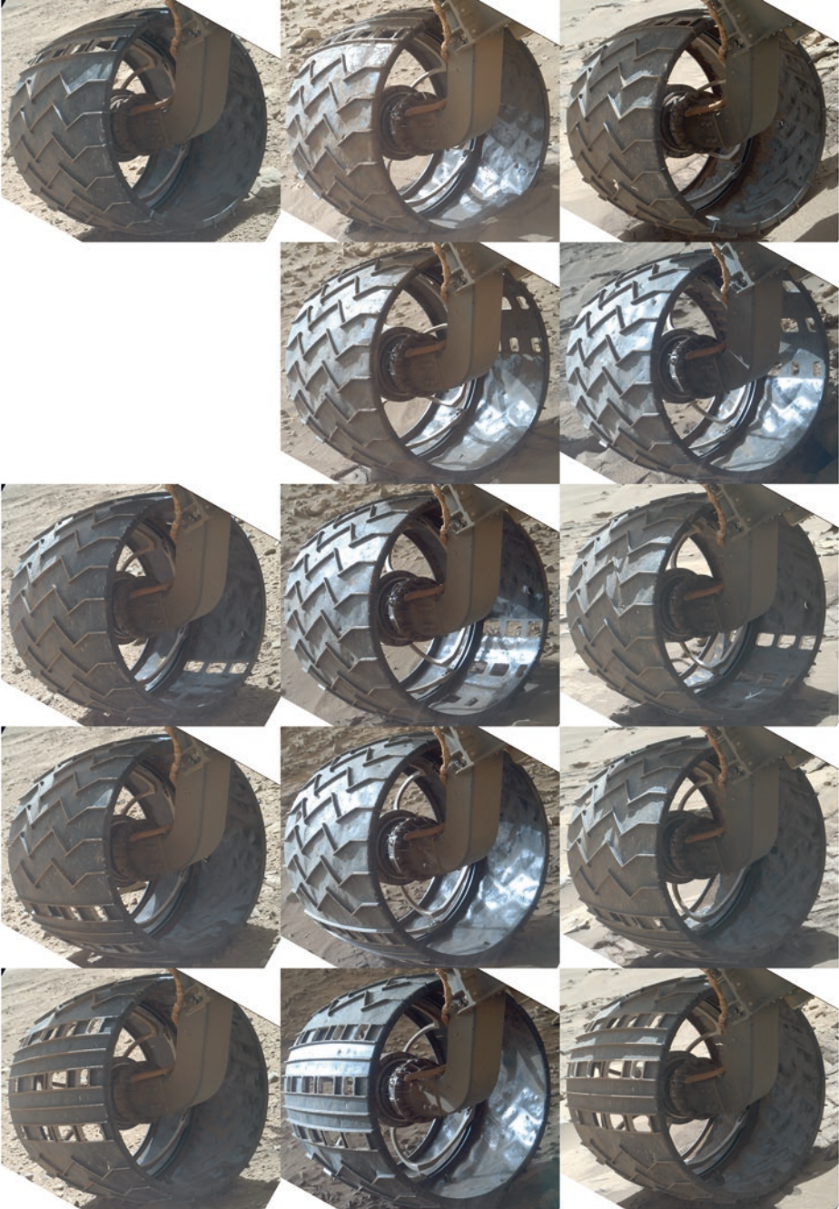
Figure 4.18. MAHLI survey of right front wheel on sol 513 (left column), 708 (middle), and 1313–1315 (right). See text for discussion. NASA/JPL-Caltech/MSSS.
