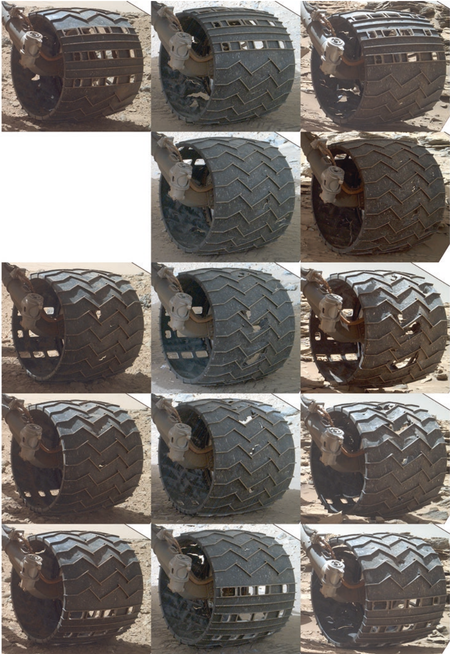
Figure 4.21. MAHLI survey of left middle wheel on sol 513 (left column), 708 (middle), and 1313–1315 (right). See text for discussion. NASA/JPL-Caltech/MSSS.
