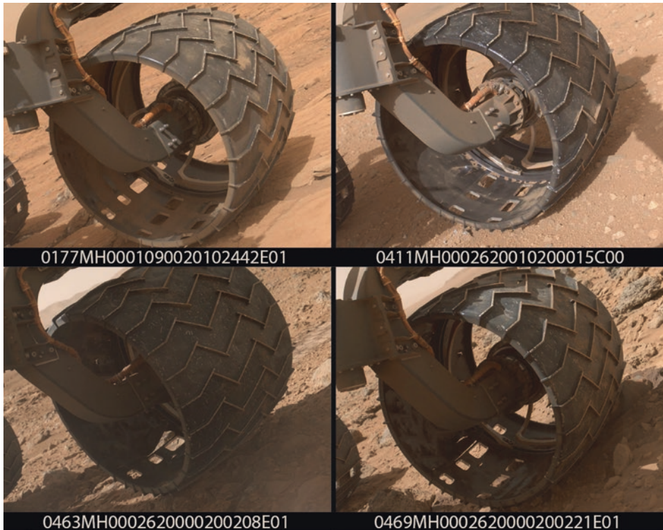
Figure 3.9. Development of damage to the left front wheel. MAHLI images taken on sols 177, 411, 463, and 469. NASA/JPL-Caltech/MSSS.
