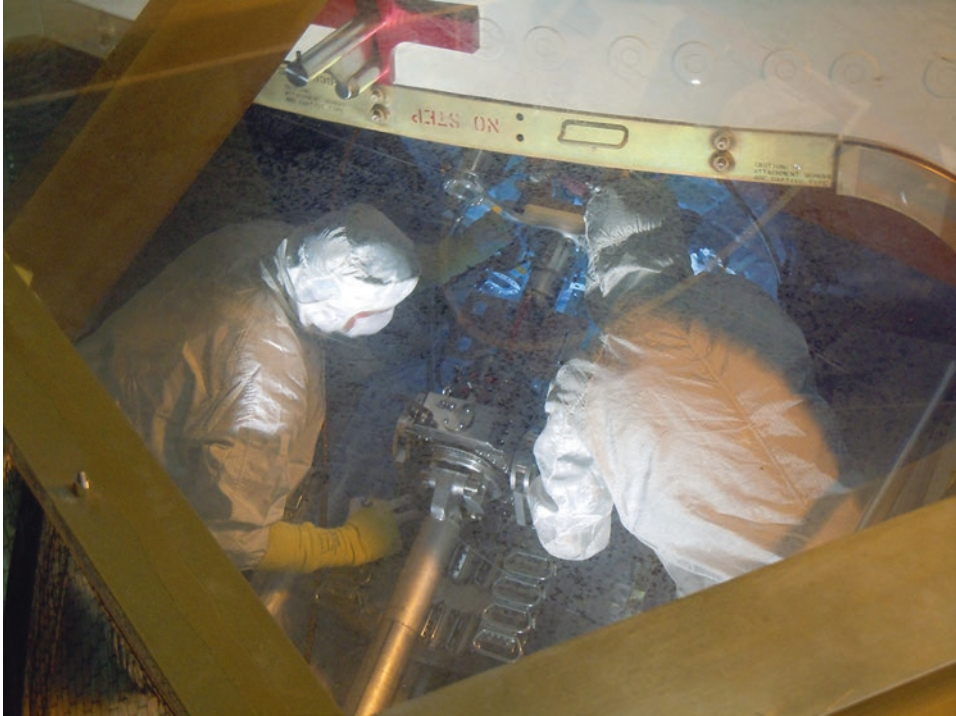
Figure 1.27. Engineers work through a hatch in the rocket fairing and a second hatch in MSL's backshell to install the MMRTG onto the rover, November 17, 2011. NASA/KSC release KSC-2011-7900.
