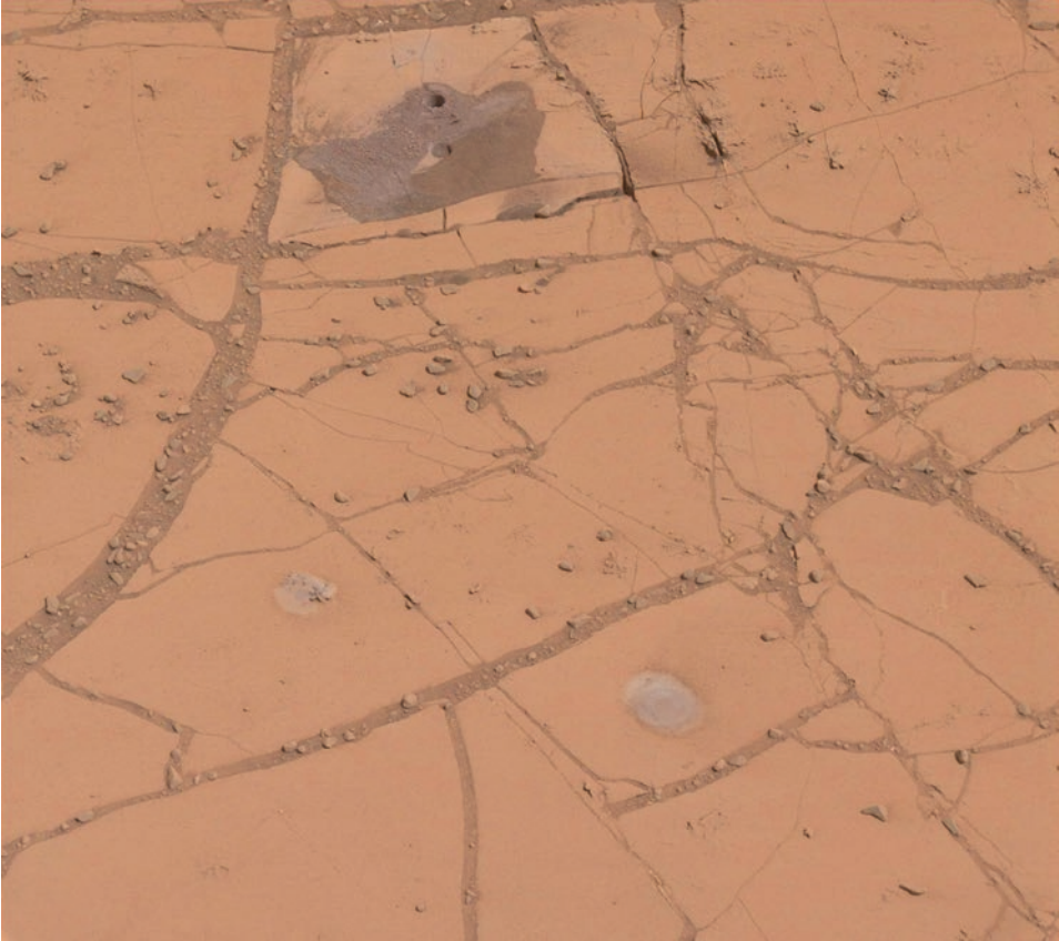
Figure 5.16. Moenkopi (left), brushed on sol 758, was a raised feature. Maturango (right), brushed sol 755, was a flat spot, and the brush was moved during brushing. The Confidence Hills drill site is in the background. Drill holes are 16 mm across; brushed spots are at least 45 mm across. Left Mastcam image 0758MH0001900010204611C00. NASA/JPL-Caltech/MSSS.
