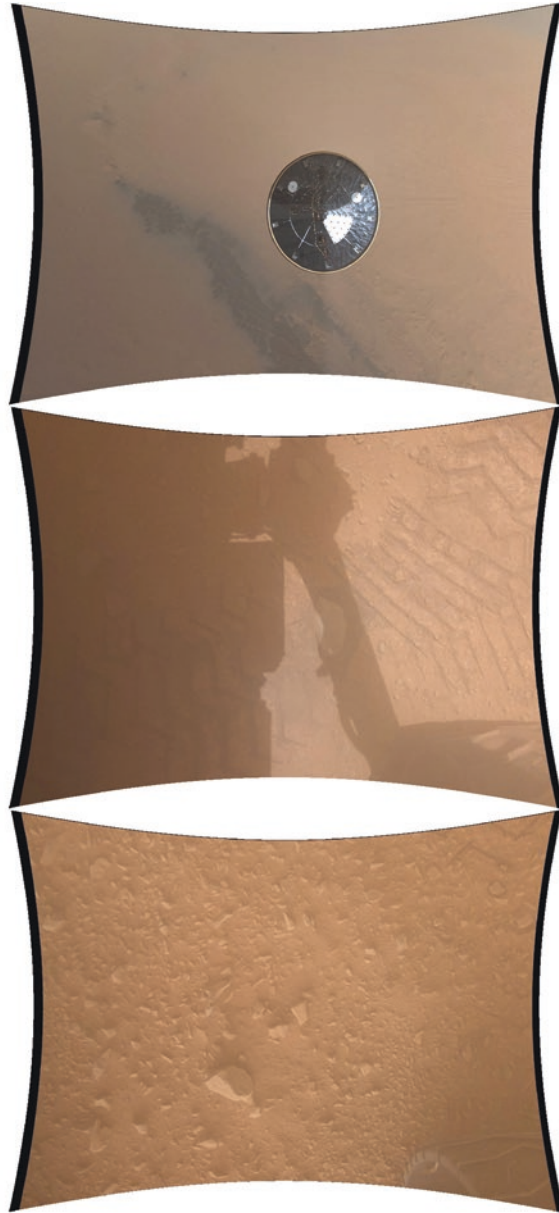
Figure 7.10. Examples of MARDI images. Top: View of the heat shield during descent. Middle: sol 45 image under daylight conditions, showing reduced contrast. Bottom: sol 738 image under twilight conditions, which improves contrast. Images 0000MD000000000100035C00, 0045MD0000300000101520E01, and 0738MD0003120000102267E01. NASA/JPL-Caltech/MSSS.
