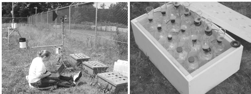
Figure 5. Outdoor tests showing Buchner funnels used to hold the HE pieces. Any precipitation landing in the funnel moves through the glass frit and into 1-L glass bottles in the wooden boxes.
