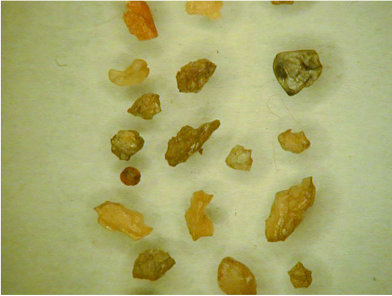
Figure 2. Example of 2,4,6-trinitrotoluene (TNT) particulates found in military impact areas from a low-order detonation.
