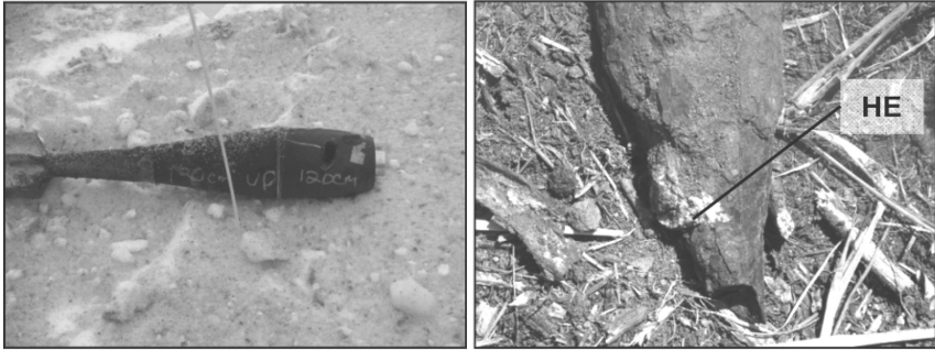
a. 81-mm round pierced by a fragment from a high-order detonation
