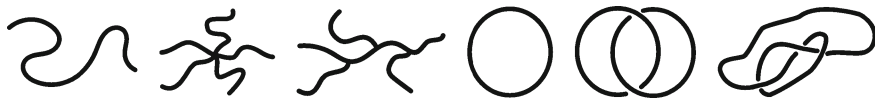
Fig. 1.2 Polymers with different topologies. From left to right : linear, star, branched (quenched), circular or ring, linked and knotted
