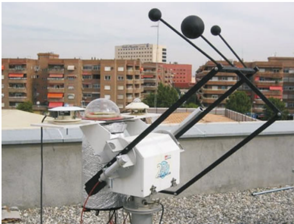
Fig. 24.4 An All Sky Imager (ASI) installed on a rooftop at Grupo de Física de la Atmósfera, Granada, Spain. The black arms with three black spheres compose the Sun tracker. The biggest central sphere shades the fisheye lens of the ASI, while the two smaller ones on the sides shade two other optical instruments placed nearby the ASI on the same platform (source of the photograph: http://atmosfera.ugr.es/inv/index.php/es/instrumentacion/76-all-sky-imager.html )
