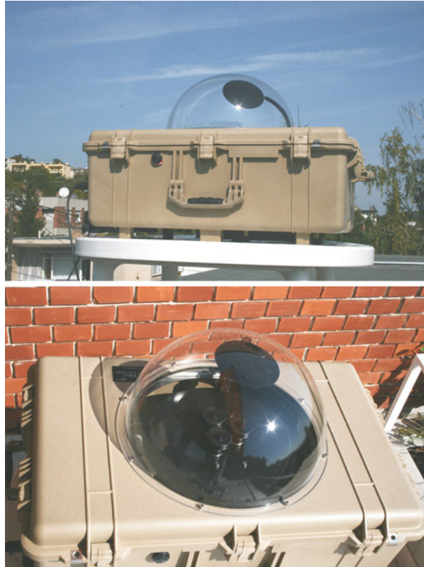
Fig. 24.6 Full-Sky Imaging Polarimetric Cloud Detector (FSIPCD) developed by the Estrato Ltd tested in the expedition ANT-XXVII-1-2010 from Bremerhaven (Germany) through the Atlantic Ocean to Capetown (South Africa) onboard the research vessel Polarstern organized by the German Alfred Wegener Institute for Polar and Marine Research (Barta et al. 2014). Underneath the transparent dome, the fisheye lens and the arbitrarily adjustable solar occulter are visible
