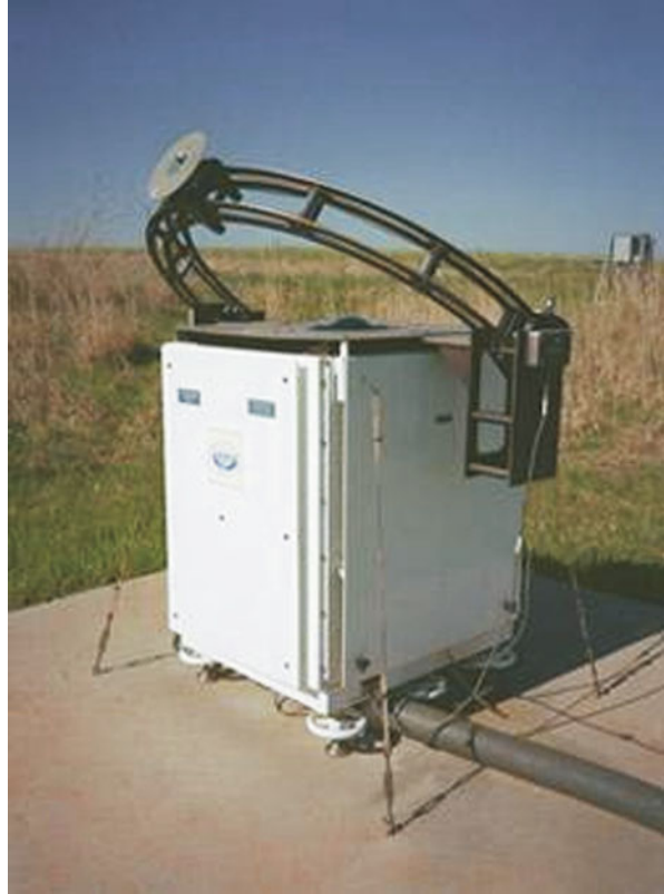
Fig. 24.2 A Whole Sky Imager with the solar occulter trolley and arc system (source of the photograph: http://www.arm.gov/instruments/wsi )
