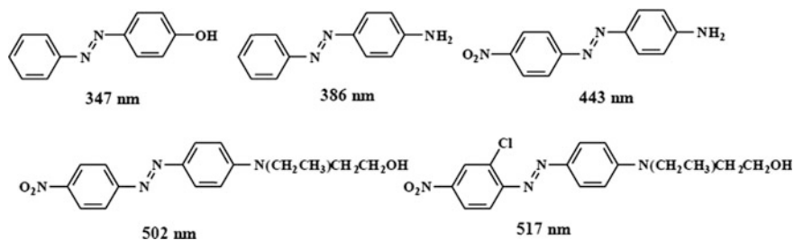
Schema 2.5 Effects of substituent groups within an azo-dye system. Reproduced from IARC, Copyright 2010, with permission from WHO
