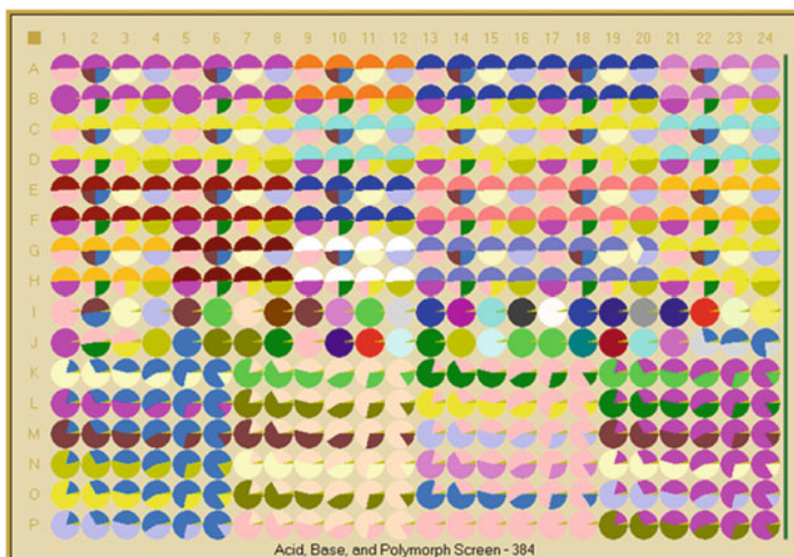
Fig. 7.12 Example of a 384-well screening design matrix aimed at discovery of acid and base salts, co-crystals, and polymorphs. Different colors represent different components within the well
