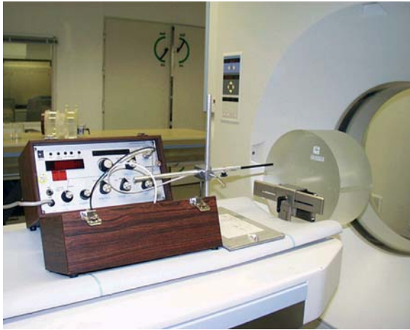
Fig. 4.44. Dose measurements in CT. The equipment consists of a 100-mm-long ionization chamber and a 32-cm Lucite phantom. With this set-up, the CTDI_w value for the body is determined
