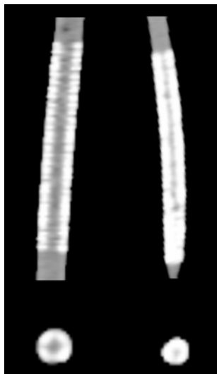
Fig. 7.39. In vitro imaging (4-slice CT, 0.5-mm detector collimation) of stents in contrast-enhanced silicon tubes: Synthesis Star 4.0 and 3.0 mm (CardioVascular Dynamics, Irvine, USA). While the magnitude of the blooming effect seems similar in both stents, only a very limited area of relatively artifact-free lumen remains in the 3.0-mm stent
