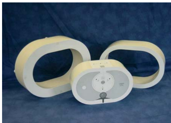
Fig. 4.51. Anthropomorphic calibration phantom (QRM Quality Assurance in Radiology and Medicine GmbH, Möhrendorf, Germany) recommended by the International Consortium for Standardization in Cardiac CT. The original phantom can be used with up to two additional attenuation rings to simulate small, medium-sized, and large patients
