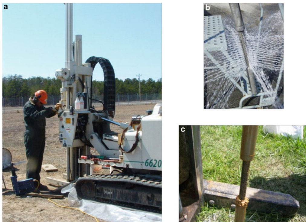
Figure 11.4. Photos of a direct-push technology rig and tooling.
