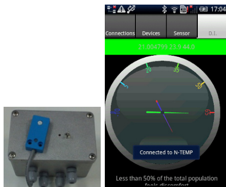
Fig 1. The environmental sensor (left) and a screenshot of the user application (client side, right) that have been implemented for the PESQoL system in Thessaloniki, Greece
