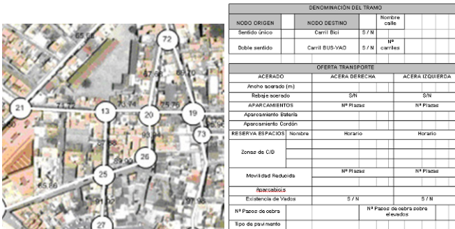
Fig. 5. Digitalization of the road by a graph and data collection cards of streets.
