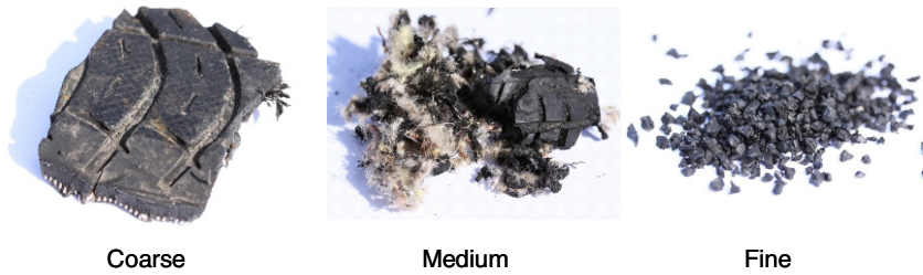
Fig. 1. Relation of particle size and liberation grade of scrap tires
