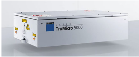
Fig. 5.9 TruMicro Series 5000 laser, delivering up to 150 W of <10 ps pulses (sub-ps with CPA) at base repetition rates between 100 kHz and 1 MHz. A flexible external modulator allows for individual pulse triggering (pulse-on-demand) via TTL input as well as fast energy modulation
