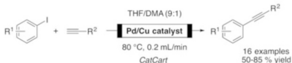
Scheme 3.4 Sonogashira coupling with Pd/Cu-mixed catalyst and basic conditions
