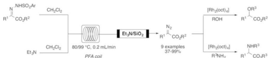
Scheme 10.7 Synthesis of \alpha -amino or \alpha -alkoxy acid derivatives via an in situ diazoester intermediate formation
