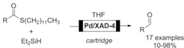
Scheme 10.21 Continuous flow Fukuyama reduction of thioesters
