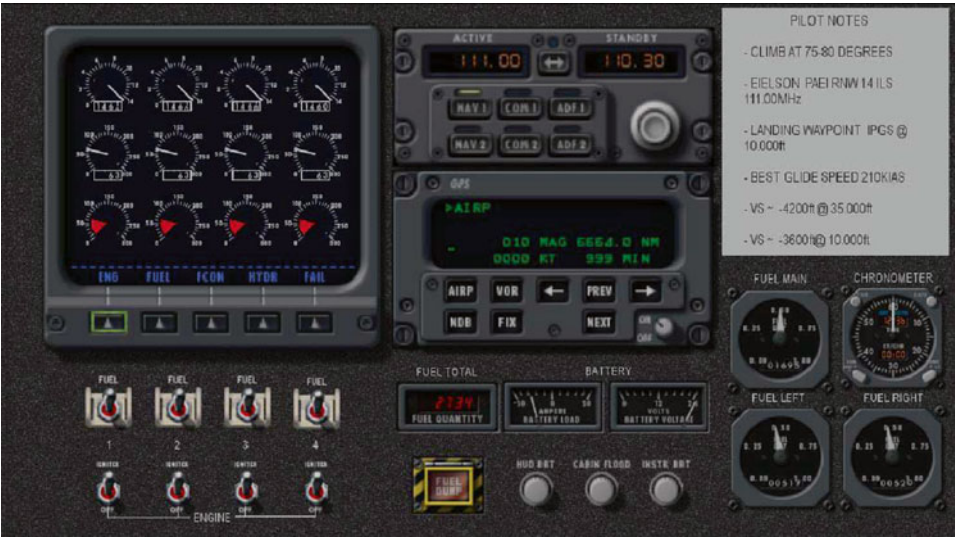
Fig. A9 Co-pilot panel with ECAM, radios and GPS, engine and fuel management buttons. Credit Vasco Ribeiro
