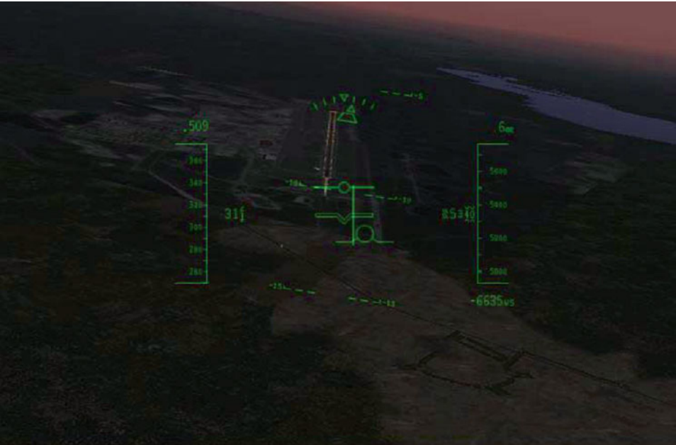
Fig. A10 Head-Up Display with speed on the left, altitude on the right, flight path vector and ILS markers on the center. Credit Vasco Ribeiro
