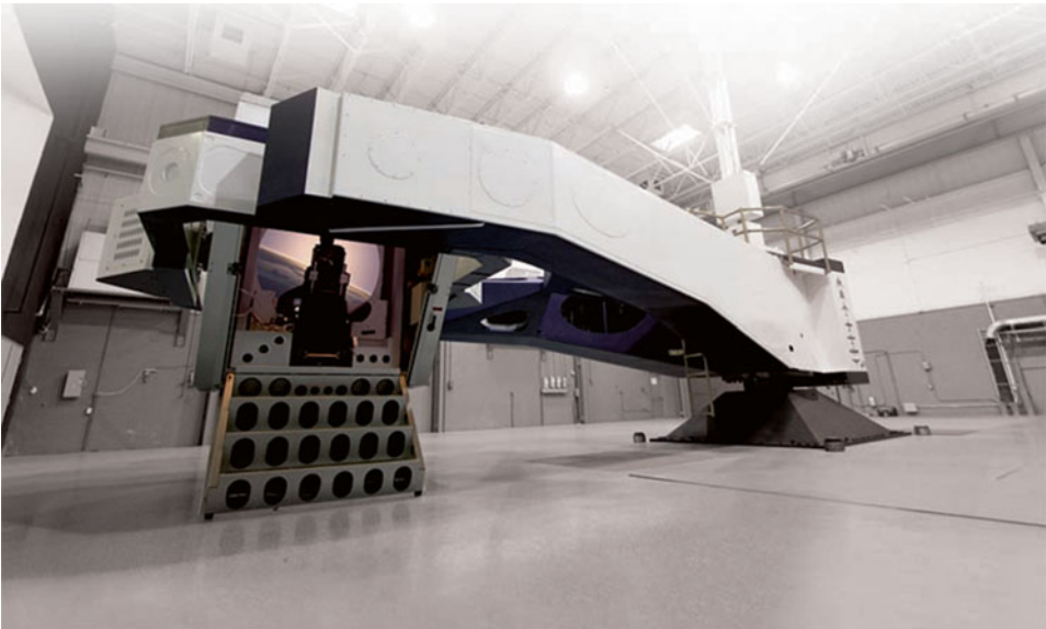
7.20 NASTAR's centrifuge: the STS-400. "Flights" in the STS-400 are preceded by classroom lectures on the subjects of acceleration and the physical effects of spaceflight. Credit: NASTAR
