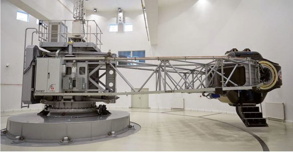
1.9 The centrifuge: equipment used to train suborbital astronauts. Credit: ESA
