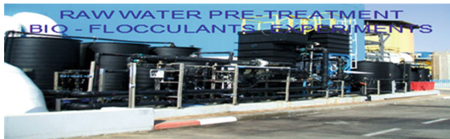
Photo 9.1 The Pilot Plant (10 m 3 /hr) used for the experiment showing the raw seawater pretreatment stage
