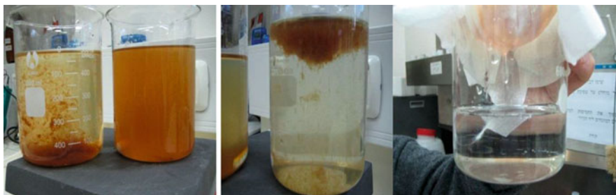
Photo 9.2 DMF backwash water before and after dosing of biofloculants and after filtration
