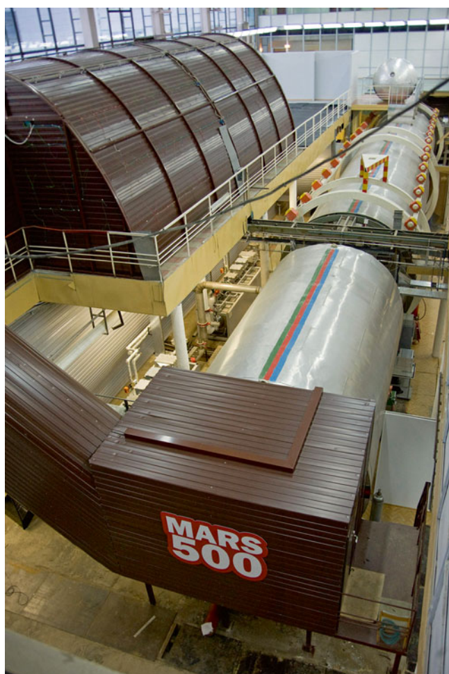
Fig. 9.9 The exterior of the Mars 500 habitats. The Mars 500 facility housed a crew for 17 months. The airlock and Mars environment are to the left (Image courtesy of Mars 500 project, © IBMP/Oleg Voloshin)
