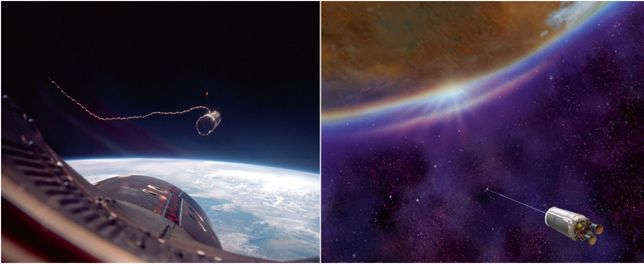
Fig. 9.7 Right: An Agena upper stage floats at the end of a tether, seen out the window of Gemini 11. The experiment was the first using tethers in a human mission to simulate gravity in space. (Image courtesy of NASA/JSC.). Left: Mission scenarios such as Robert Zubrin's Mars Direct would use tethers to imitate gravity on the long transit journeys to and from Mars (Painting by Michael Carroll, courtesy of the Mars Society)
