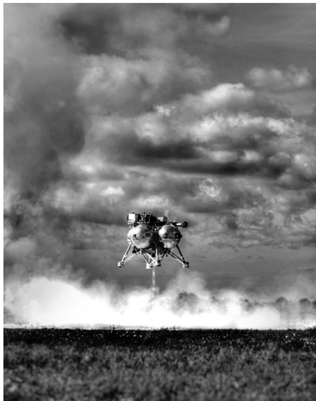
Fig. 10.12 The methane-powered Morpheus craft on a test flight at the Kennedy Space Center in Florida (Image courtesy of NASA)
