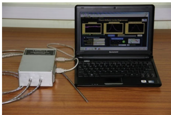
Fig. 13.8 A compact LED-based fluorescence spectroscopy system for cancer diagnosis
