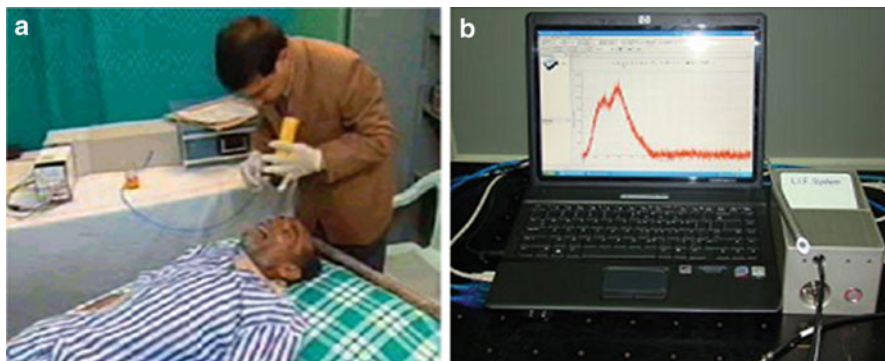
Fig. 13.6 (a) The first prototype nitrogen laser-based fluorescence spectroscopy system for cancer diagnosis (b) a more compact version of the fluorescence spectroscopy system
