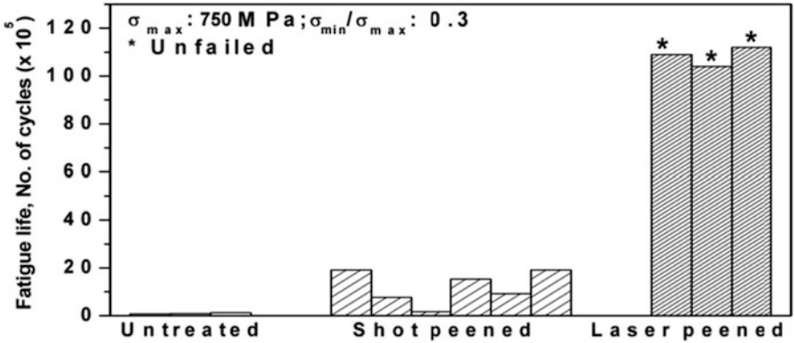
Fig. 12.16 Comparison of fatigue lives of untreated, shot-peened, and laser-peened specimens of SAE 9260 spring steel
