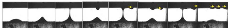
Fig. 12.10 Combination of the dispensing function with the transportation of the droplets. The angle in this case is clearly visible in the picture and is \sim 11^\circ with respect to the normal to the substrate
