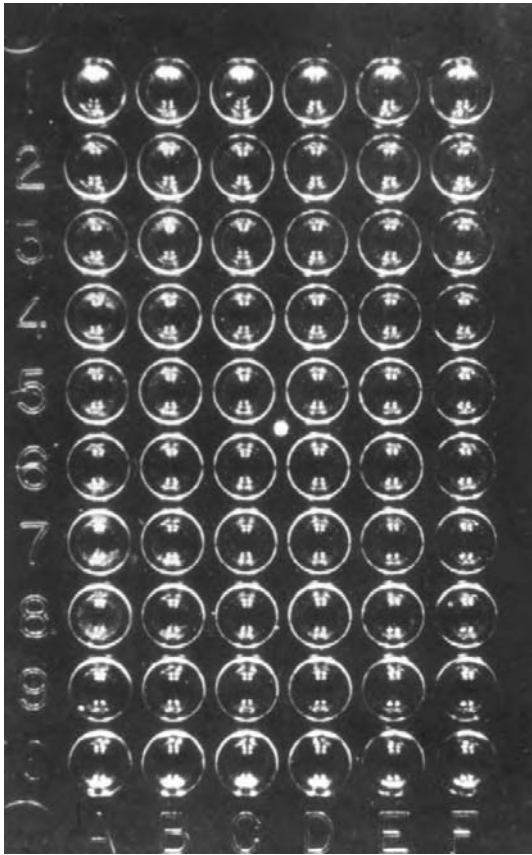
FIGURE 21.11 A Terasaki plate consisting of depressions in a plastic plate that contains pre-disposed antibodies to HLA antigens of various specificities and into which are placed patient lymphocytes and rabbit complement for tissue typing.
