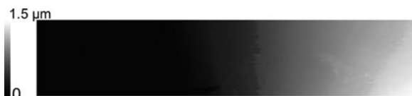
Fig. 7 Height as calculated by the model is mapped in gray scale for each point in the marked area in the images. The size of the image is 140 \mu\text{m} \times 28.2 \mu\text{m}
