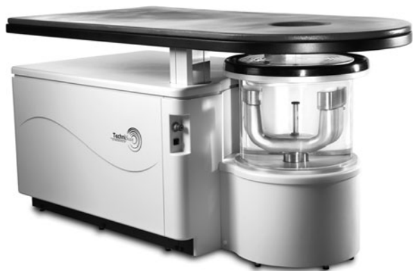
Fig. 1 TMS, Inc. Whole Breast Ultrasound (WBU) clinical device
