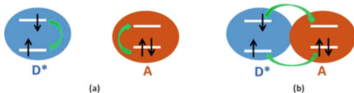
Fig. 3.7 Schematic representation of FRET (a) and Dexter (b) ET mechanisms from an excited Donor (D) to an Acceptor (A)
