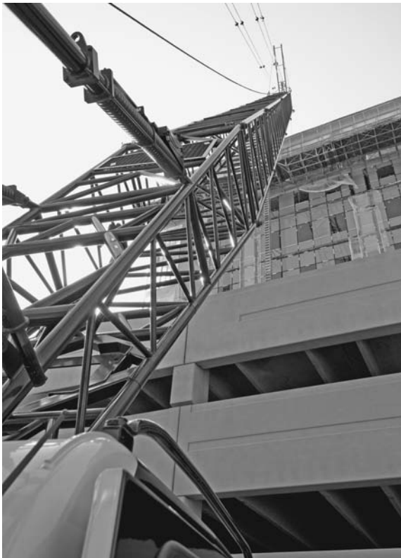
FIGURE 5.9 The operator cannot judge clearance well from the cab. A well-placed signalperson with a dedicated radio link to the cab is advisable. ( Link Belt Construction Equipment Company. )
