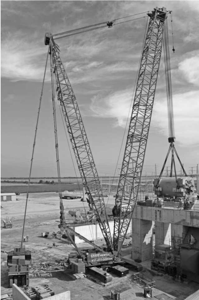
FIGURE 2.28 A Manitowoc 2250 crawler crane with a proprietary wheeled counterweight tray and a live mast. The wheels are shown oriented for slewing , but they can also be repositioned for travel. (Manitowoc Company, Inc.)
