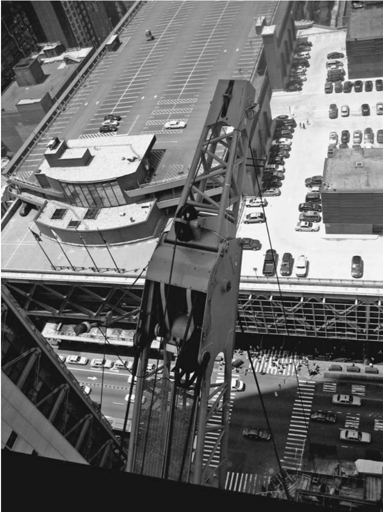
FIGURE 2.18 Rooster sheave on a boom tip above Times Square in New York City. Main and auxiliary hoist lines are visible. (Lawrence K. Shapiro.)
