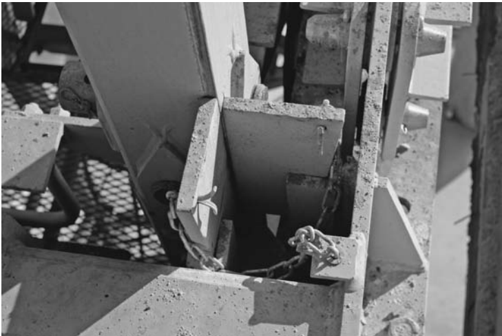
FIGURE 6.37 Wedging arrangement that is part of a climbing base. ( Manitowoc Corporation Inc. )
