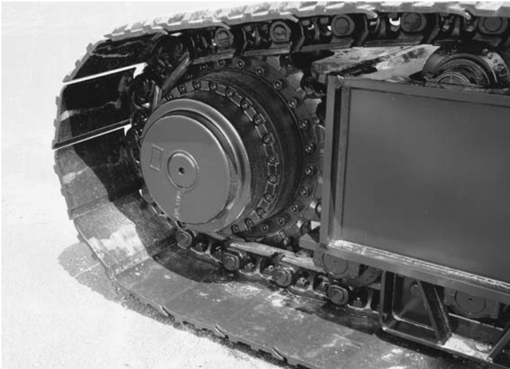
FIGURE 2.11 The crawler is propelled by a hydraulic motor at the rear end of the side frame, mounted on a gearbox and powering the drive sprocket. The idler wheel at the top right maintains tension in the track. Track rollers are on the bottom. (Link Belt Construction Equipment Company.)
