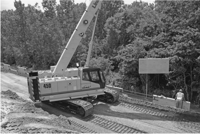
FIGURE 2.30 Once a rarity, a telescopic boom mounted on a crawler base is not uncommon for site work, particularly pick and carry. (Link Belt Construction Equipment Company.)
