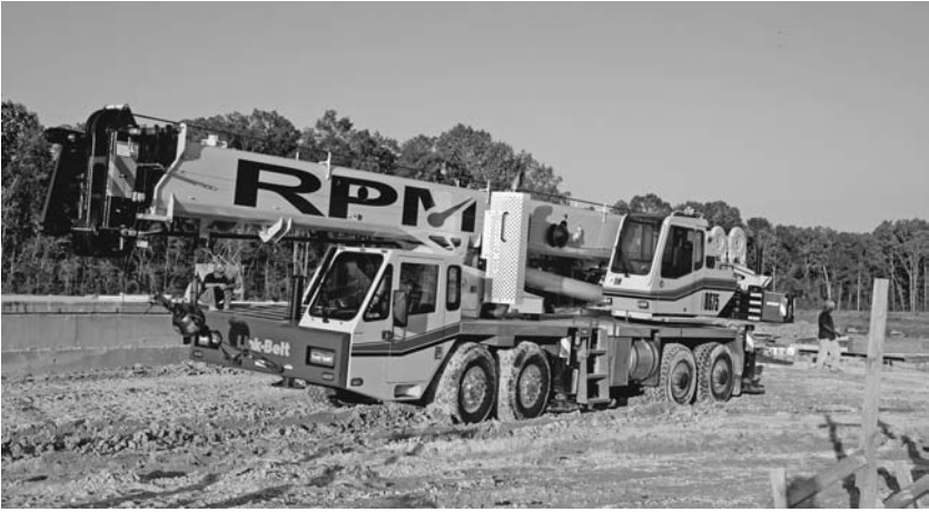
FIGURE 2.14 A 90-ton all-terrain hydraulic truck crane moving off road. Characteristics of all-terrain cranes include high road speed, off-road maneuverability, pick-and-carry ratings, all-wheel drive and steering, crab steering, and driving controls in both the carrier and the upper cabs. (Link Belt Construction Equipment Company.)
