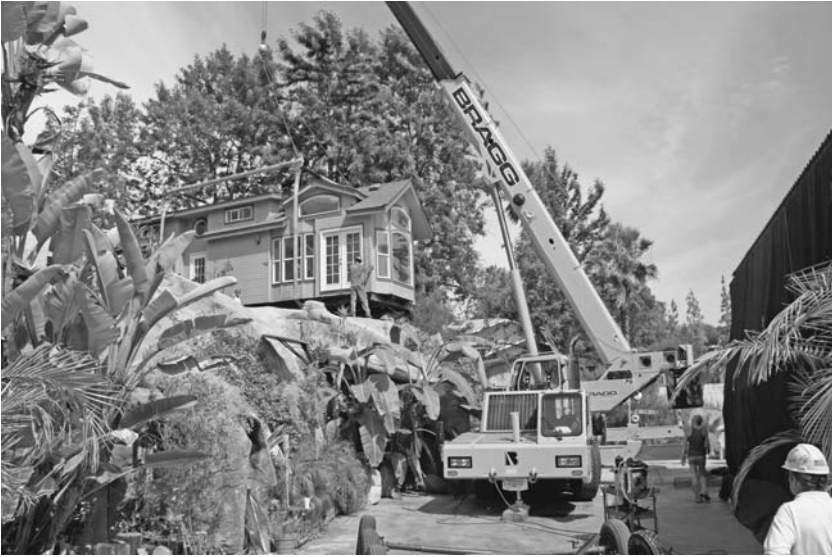
FIGURE 4.6 Telescopic truck crane with a front outriggers that allows the crane to operate in a full circle. ( Link Belt Construction Equipment Company .)
