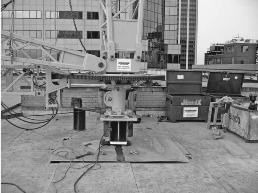
FIGURE 7.31 Bull wheel used to swing a stiffleg derrick. It is driven by a chain connecting the bullwheel to a smaller sprocket driven by a hydraulic motor. The footblock, mounted directly to the top of a building column, has a pair of sheaves to lead the load hoist and boom hoist lines. ( Budco Rigging Co. )
