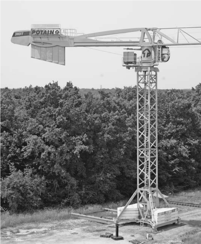
FIGURE 6.4 Tower crane freestanding on a chassis base with concrete ballast. The base must be supported on a competent bearing surface. (Manitowoc Company Inc.)
