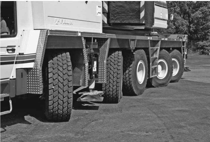
FIGURE 2.15 Crab steering on a 200-ton all-terrain crane. (Link Belt Construction Equipment Company.)
