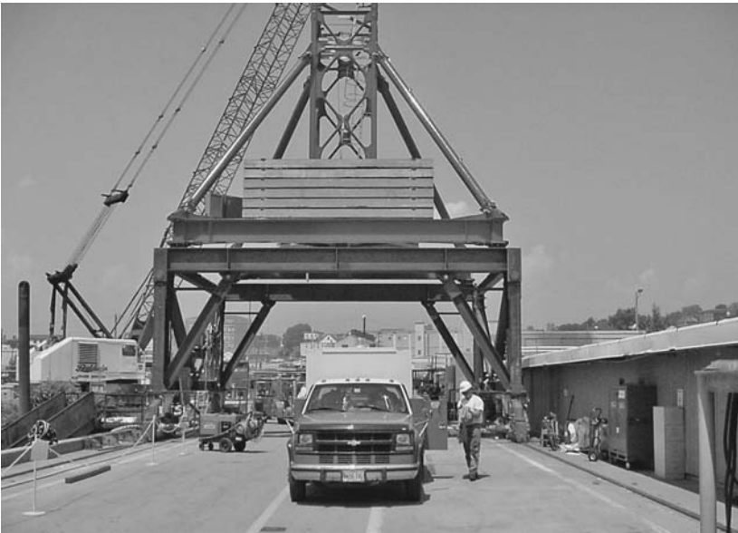
FIGURE 2.45 Traveling portal-mounted tower crane. The portal mount permits the crane to pass over materials or vehicles between the tracks. ( Manitowoc Company, Inc. )
