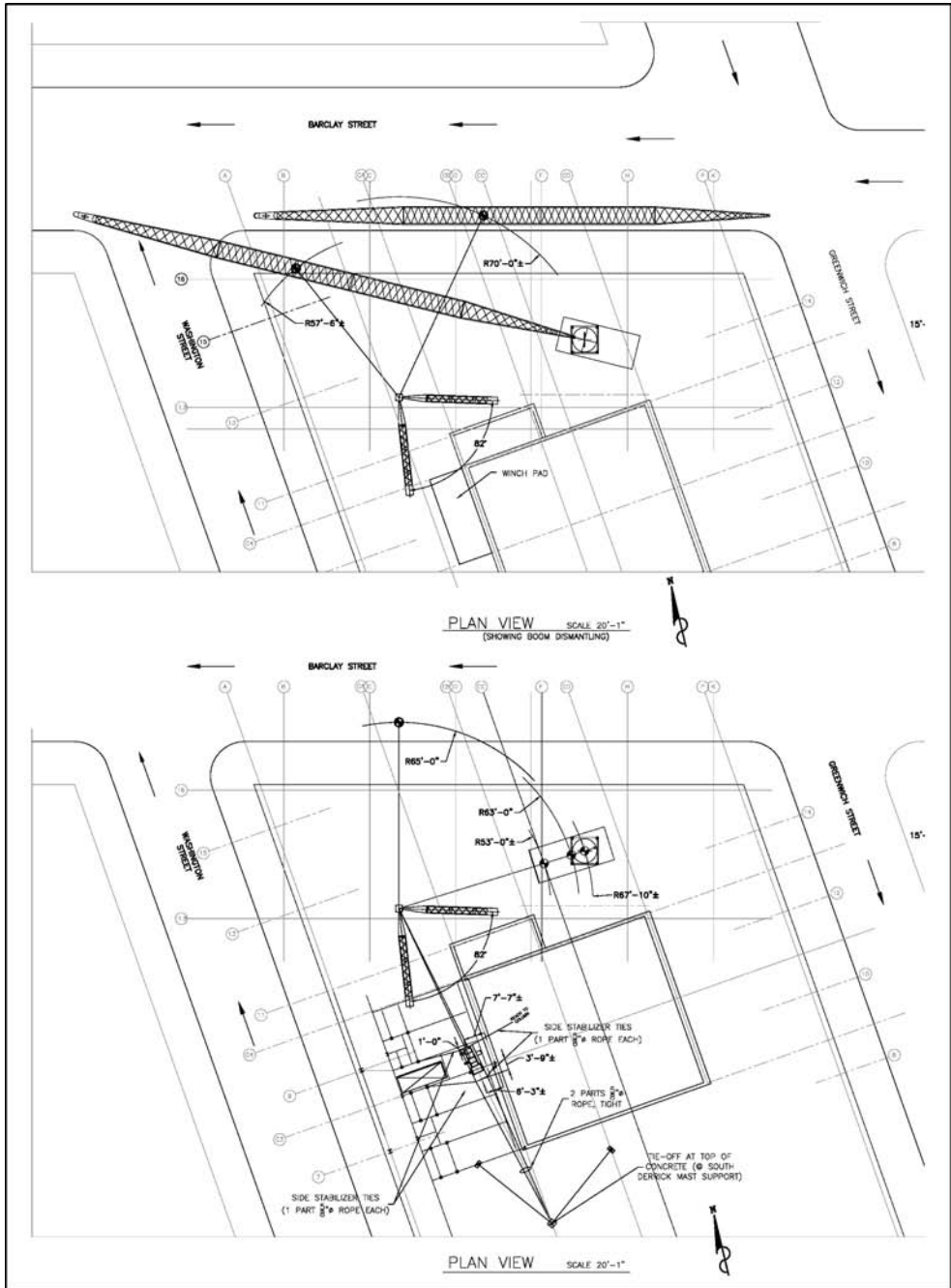
FIGURE 7.30 (b) This sheet shows the winch mounting and the procedure for dismantling the tower crane.
