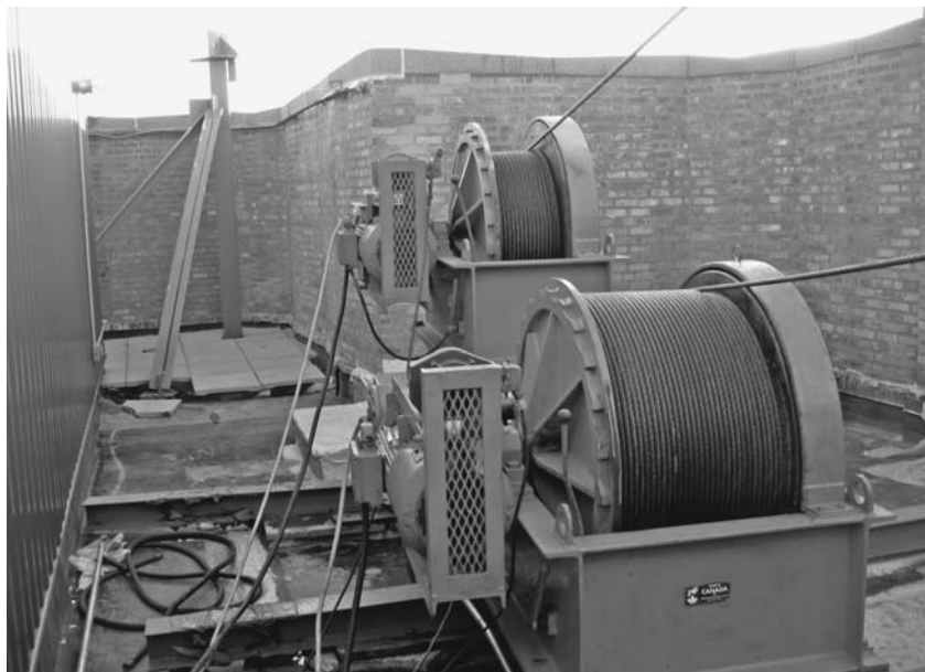
FIGURE 7.40 Dual drum winch designed for derrick work on existing buildings. Its weight is spread out on the roof by steel dunnage. Narrow drums allow the winch to be positioned close to the footblock. This winch breaks down into pieces that are small enough for most stairwells, doorways and freight elevators. ( Budco Rigging Co. )
