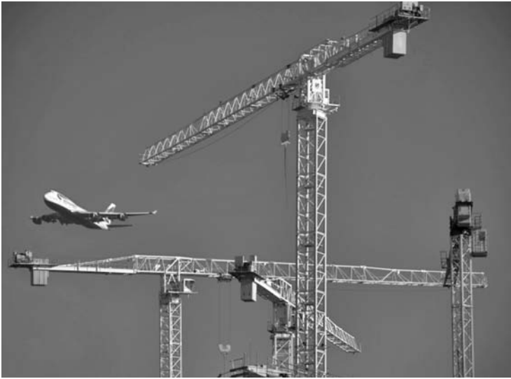
FIGURE 2.36 A Cluster of flattop-style tower cranes near an airport flight path. The tower heights are offset so that the hook of one crane can clear over the jib and counterjib of another. All the cranes must be free to weathervane when not in use. ( Terex Comedil. )
