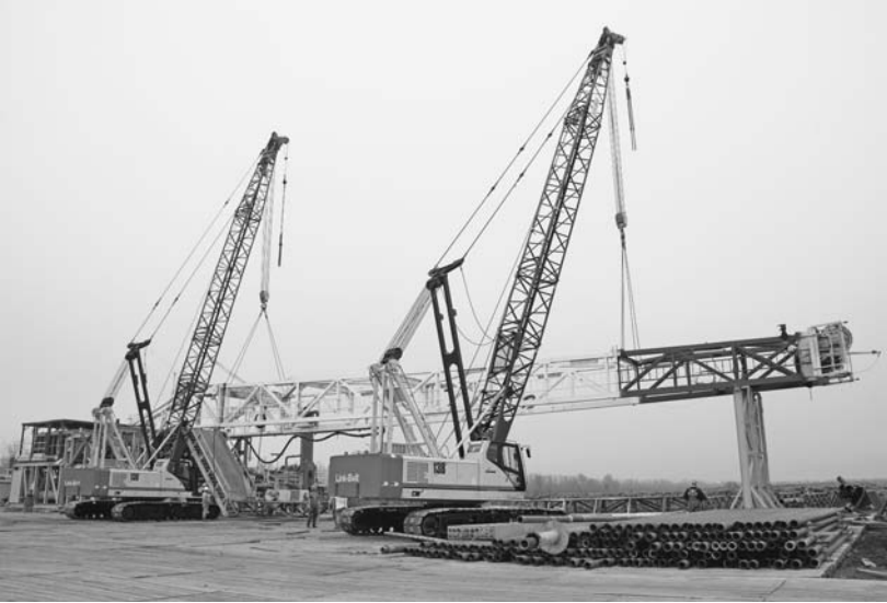
FIGURE 2.19 The live mast on these crawler cranes serves to increase the angle between the boom and the boom guy lines, and thus reduce the compressive force in the boom and increase structural capacity. ( Link Belt Construction Equipment Company. )
