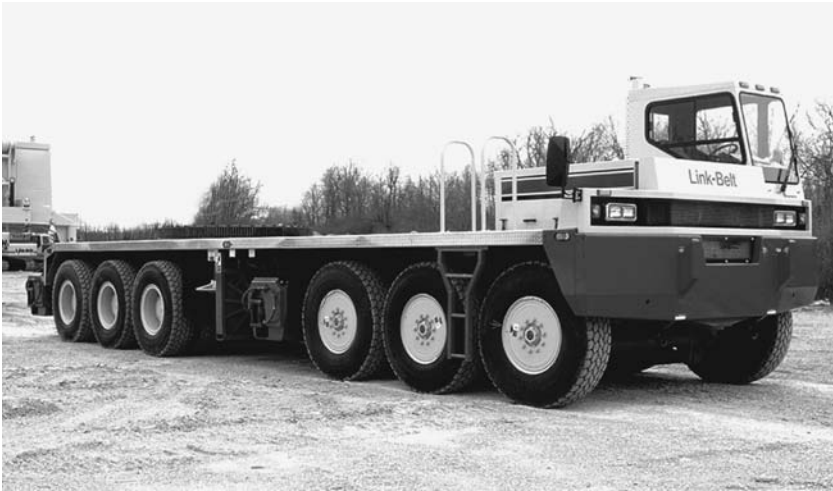
FIGURE 2.13 Carrier for a Link Belt HC-278H truck crane. (Link Belt Construction Equipment Company.)
