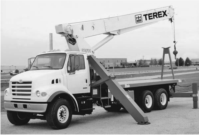
FIGURE 4.3 A boom truck is a telescopic boom joined to a truck chassis, with stabilizers. These machines are frequently used to deliver materials to an upper floor or inside a site. The stabilizers do not raise the wheels off the ground. (Terex Corporation.)
