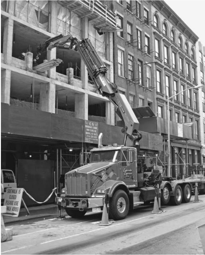
FIGURE 2.1 Articulating boom, commonly referred to as a knuckle boom, is useful for deliveries and for reaching between floors of an open building. (Lawrence K. Shapiro.)
