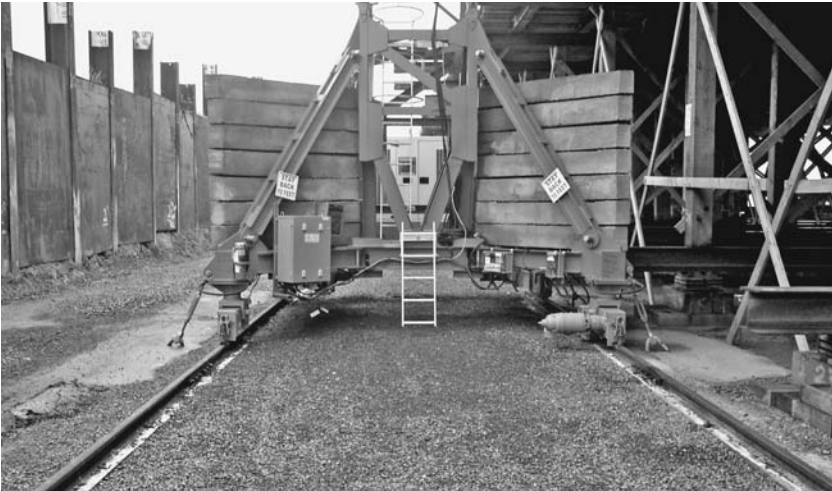
FIGURE 2.42 A travel base of a tower crane, with a knee-braced chassis and ballast weights on bogies and rails. The crane is on a parking section of track anchored down in preparation for a storm. ( Manitowoc Company, Inc. )
