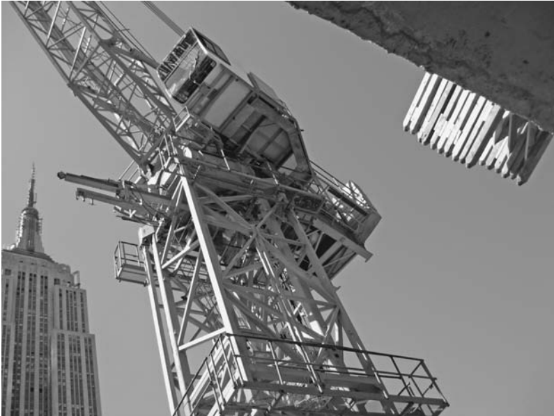
FIGURE 6.21 Climbing frame for a Liebherr 550 HC tower crane in the retracted position. The projecting trolley beam is used to carry a tower section in or out from the mast just under the turntable. Platforms are located where access is needed for operation of the equipment and making connections. ( Dominique Singh. )
