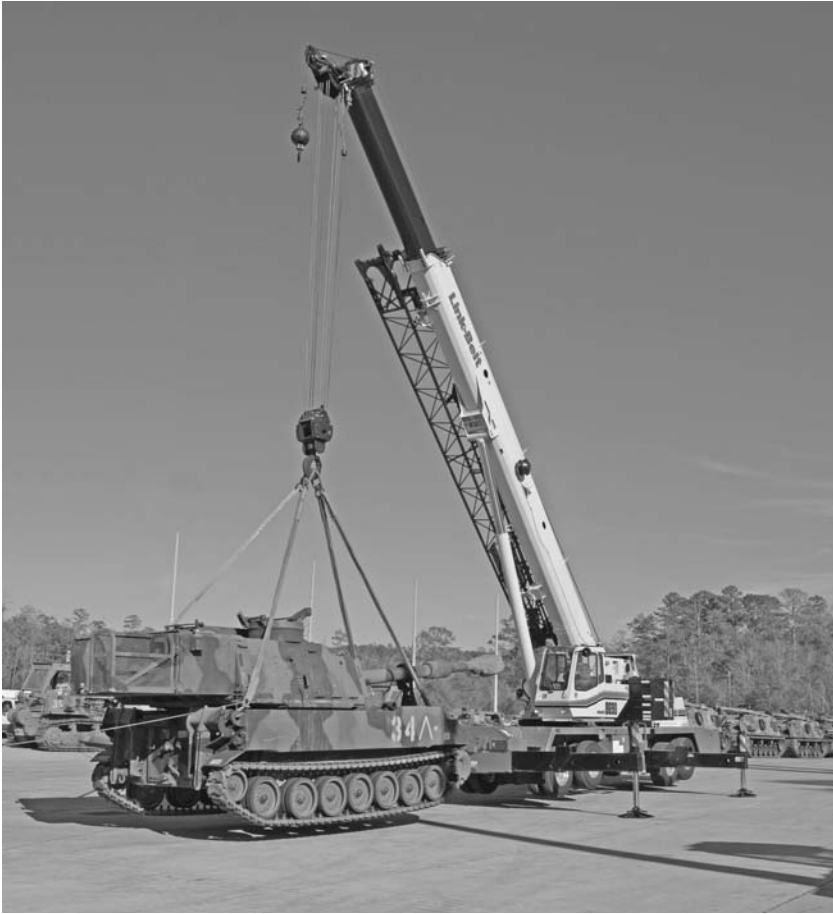
FIGURE 2.29 A 90-ton hydraulic truck crane lifting a military vehicle. The swing-away jib is stowed on the side of the boom. Lifting is from a block suspended from the main fall while the whip line is idle. ( Link Belt Construction Equipment Company. )
