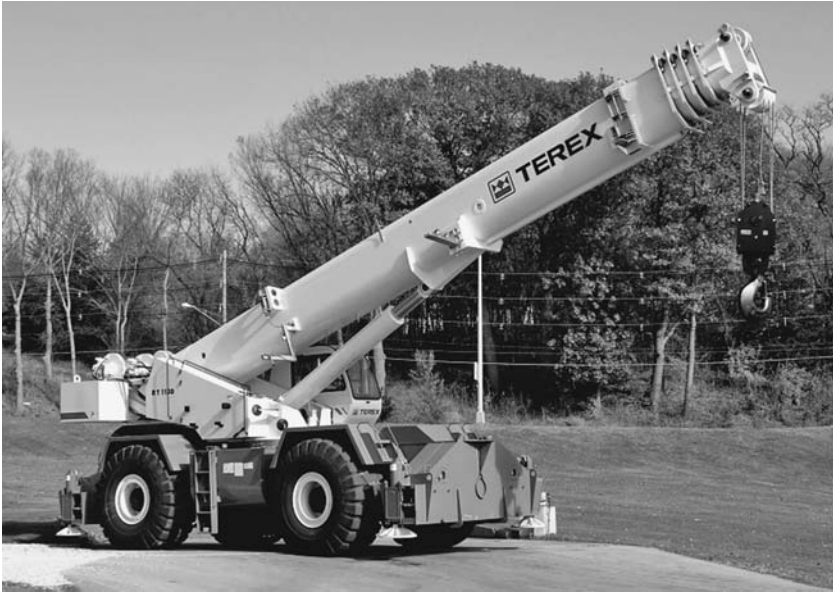
FIGURE 2.16 The unusually large wheels on this rough-terrain crane make maneuvering easier on uneven ground. Driving and operating functions are controlled from one station. (Terex Corporation.)
