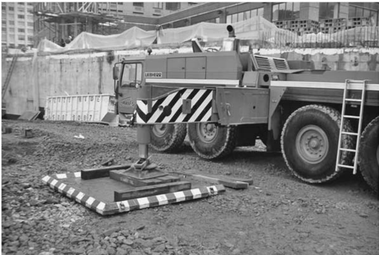
FIGURE 4.2 Outrigger on a telescopic crane with a hydraulic ram at the outboard end of its outrigger beam. After the beam is extended by means of a concealed ram, the vertical end ram is activated to raise and level the crane. The wheels of the crane must be completely elevated above the ground for the outriggers to be fully effective. ( Lawrence K. Shapiro. )
