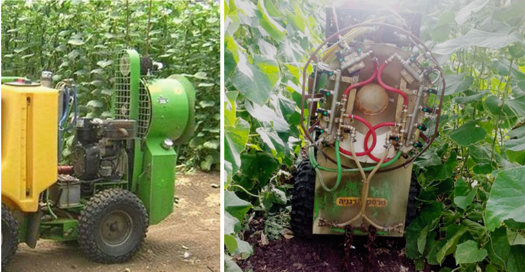
Fig. 19.3 A sprayer for cordoned crops capable of applying the spray upward for improved underleaf coverage ( left ) and equipped with electrostatic charging system ( right )
