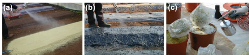
Fig. 5.5 Spray mulching coatings: a white sodium alginate; b black sodium alginate; c spray mulching application on pots
