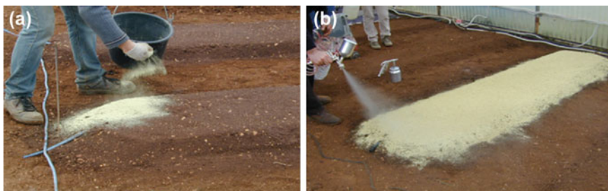
Fig. 5.11 Powder mixing deposition (a); MA solution spraying (b)
