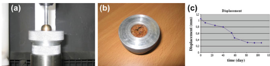
Fig. 5.12 Spherical dart (a), sample broken by dart penetration (b), curve of displacement vs time (c)
