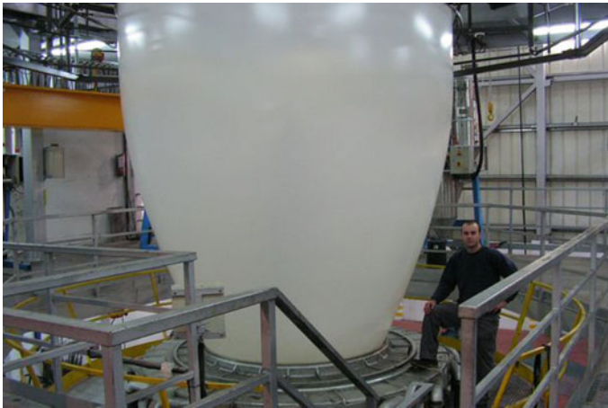
Fig. 1.3 Co-extrusion of a five-layer film for greenhouse cover the result is a multi-layer product, i.e., a product that is structured of several discrete layers, each made of a different mixture of materials and hence each layer has different properties. For example, modern greenhouse covers are typically 3–5 layer films. The outer-most layer is designed to have the best UV resistance and to reduce dust attraction. The inner-most layer is designed to prevent formation of water droplets (anti-drip) and the middle layers contribute most of the mechanical strength of the film
