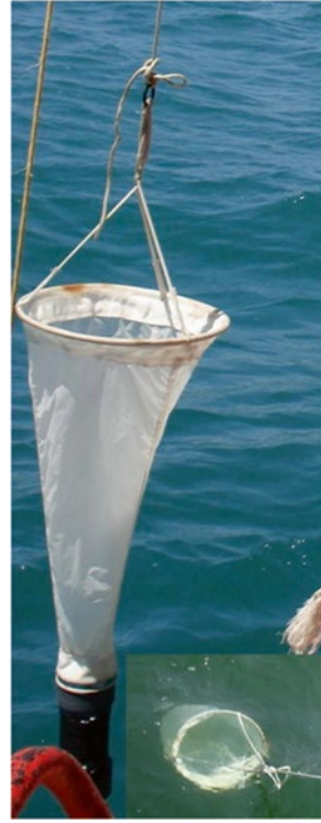
Fig. 4.4 Image of a typical phytoplankton net being hauled for phytoplankton collection (Image courtesy: www.nearhus.gr )
