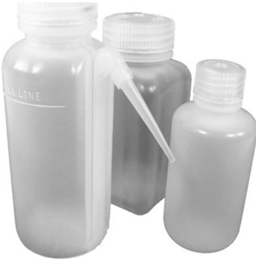
Fig. 4.1 Simple graduated bottles for collection of phytoplankton water samples. The nozzle in front allows the observer to squeeze out the measured portions of sample for study
