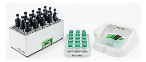
Fig. 8 Automatic methane potential test system (AMPTS) for monitoring BMP of up to 15 samples simultaneously. Material to be evaluated is mixed with an inoculum, and the gas formed is passed via a scrubber where  $CO_2$  and  $H_2S$  are removed. The remaining gas is fed to gas flow meters. Courtesy: Bioprocess Control AB, Lund, Sweden
