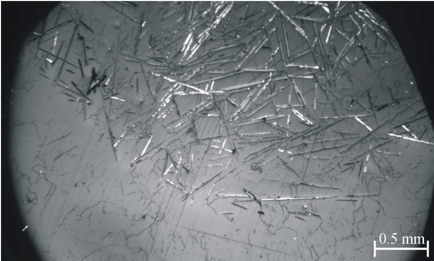
Figure 2. Etching pattern of a ZrB_{12} single crystal cross section in (100) plane from the same parts of ingot as in [23, 27, 29]. The needle like long grains are ZrB_2 phase, while the small black lines correspond to etching pits from small angle boundaries.
