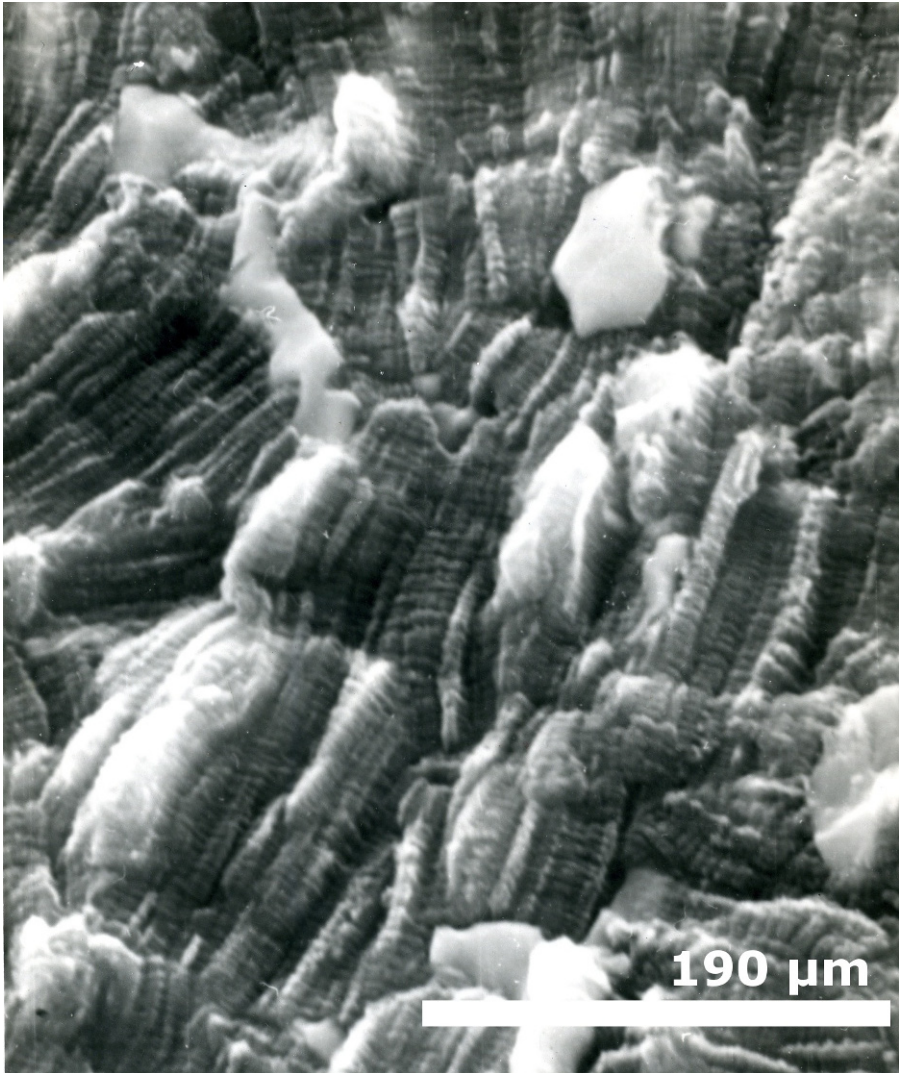
Figure 7. Stratification of RGT type graphite doped with 1%B. ( \text{He}^+ , 800 eV, T=1,300^\circ\text{C} ). The precipitates of TiC are seen on the surface.
