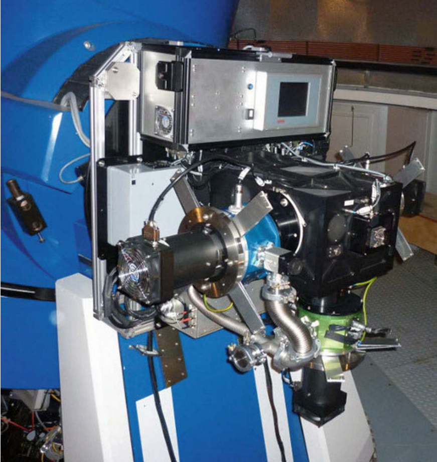
Fig. 7.4 MAIA installed at a Nasmyth focus of the Mercator telescope. The instrument consists of a black optics box, three cryostats (the blue and green coloured ones are visible on this picture, the red one sits in the back). The stirling coolers ( black with visible fan) are mounted on springs to prevent the instrument and telescope from picking up their vibrations
