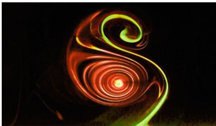
Fig. 3 Counter rotating vortex generated at the tip of a wing. (American Physical Society's 2009 Gallery of Fluid Motion)
