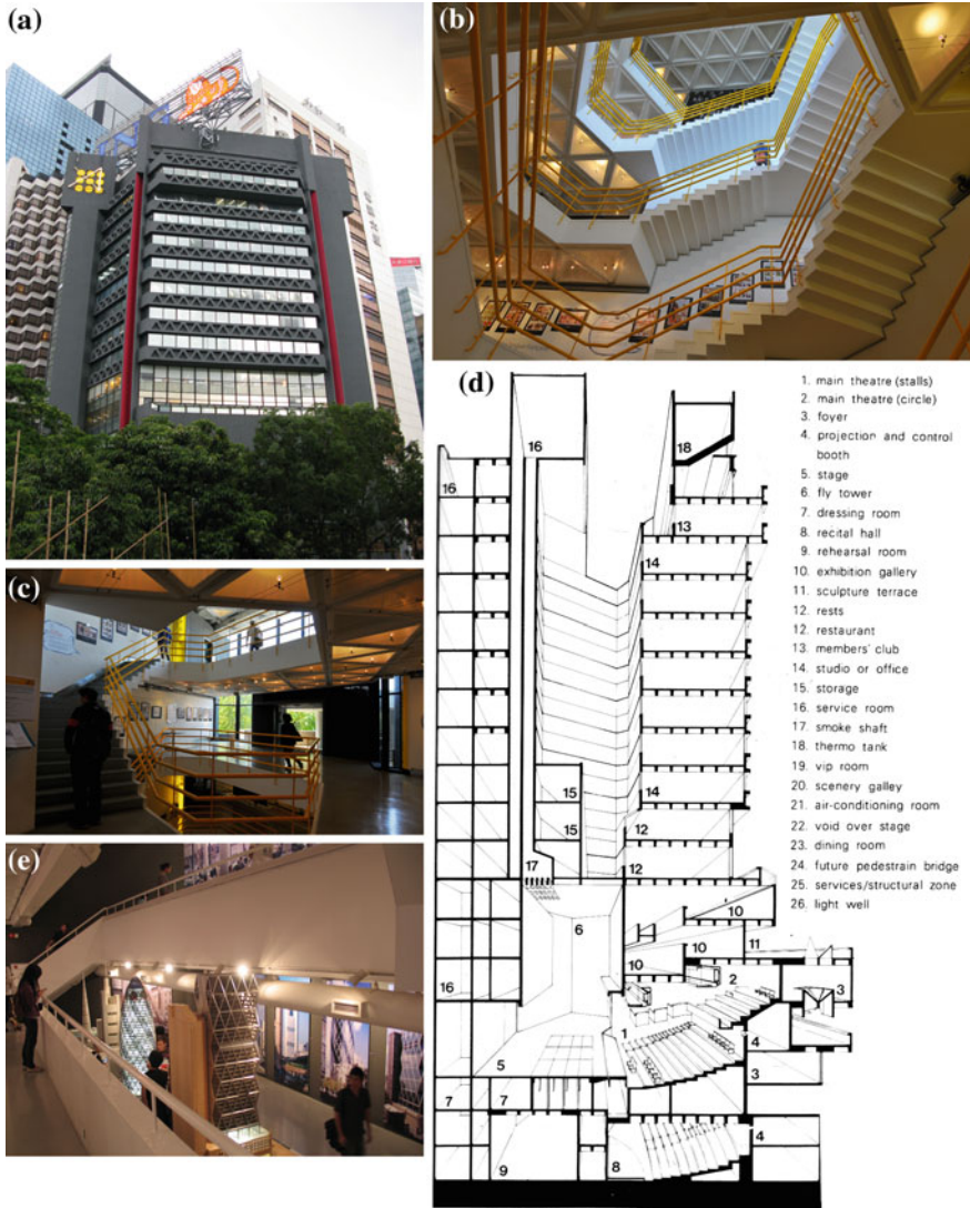
Fig. 8.11 Hong Kong Arts Center, 1977. a The main elevation facing the street corner. b Stair along the wall is the main feature of design. c The staircase dialogues with inside and outside. d Section showing the flexible usage of level heights. e Gallery. f Design sketch. Drawings courtesy of Dr. Tao Ho
