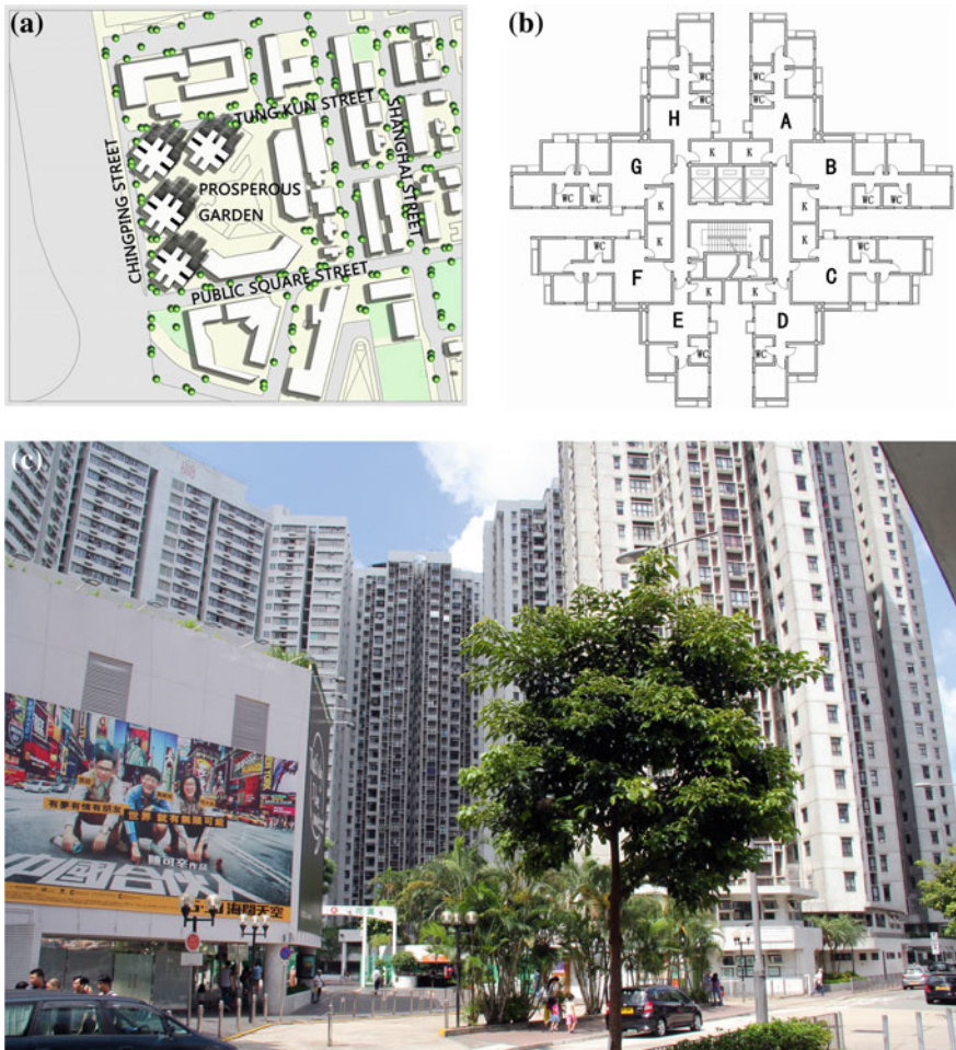
Fig. 2.8 Prosperous Garden Estate, 1995. a Master plan. b Typical floor plan. c The estate mixes rental and home-ownership blocks. Drawn by Zang Peng
