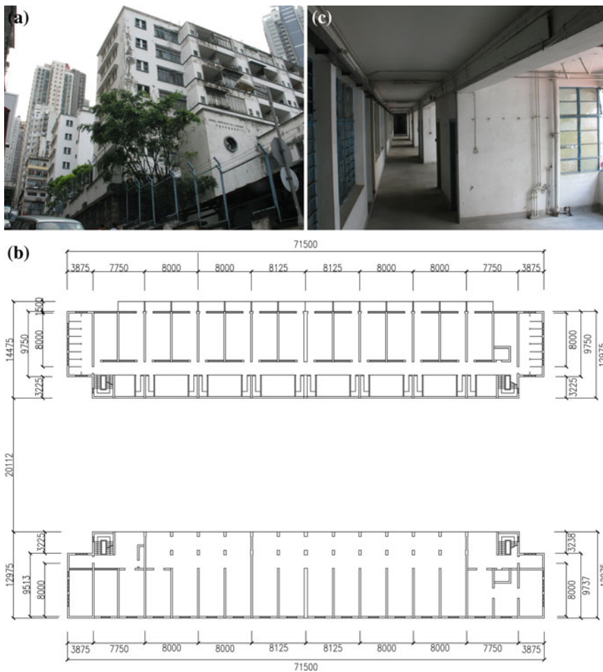
Fig. 1.8 Married police quarters, 1955. a Seen from street. b Plan. c The left hand side is living units, the right hand side is open kitchen
